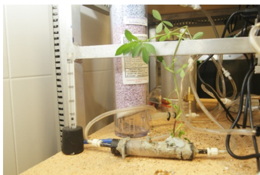
Figure 31. Apparent nitrogenase activity (ANA) estimated with an electrochemical H_2 sensor (Qubit System ® Inc., Canada). Intact alfalfa nodulated plants in the open flow system.
