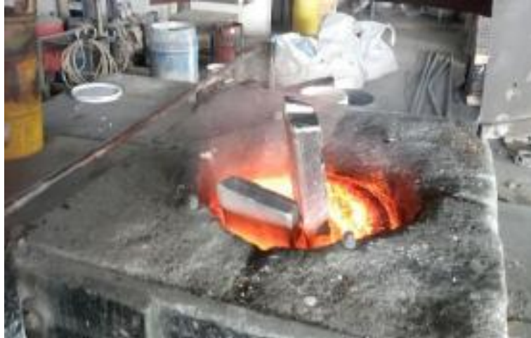
Figure 4. 1. Melting process of ingots to be used in casting works.
