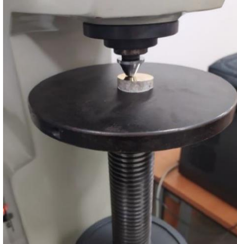
Figure 4. 2. Brinell hardness testing procedure.
