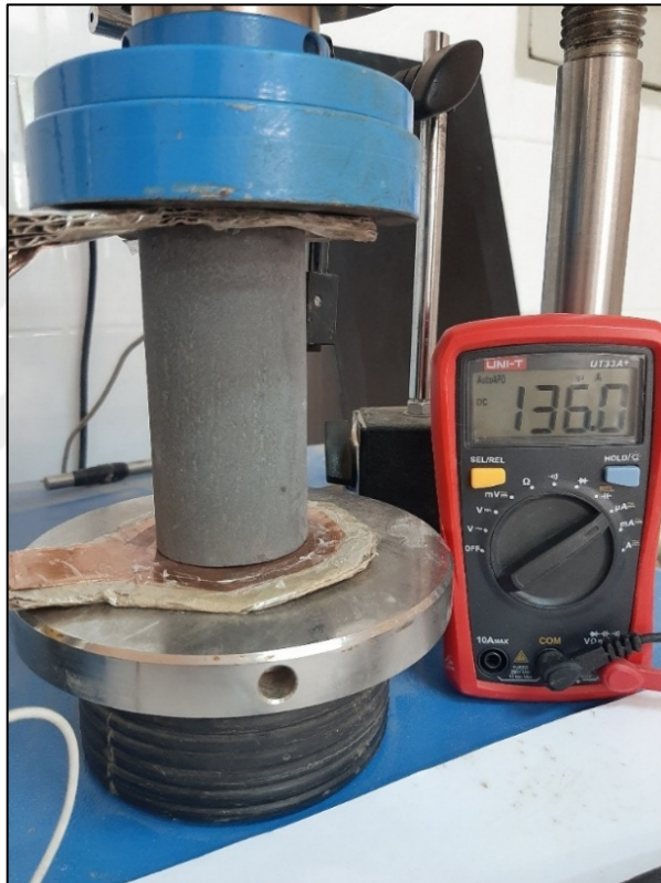
Figure 3.9 Electrical resistivity test setup
