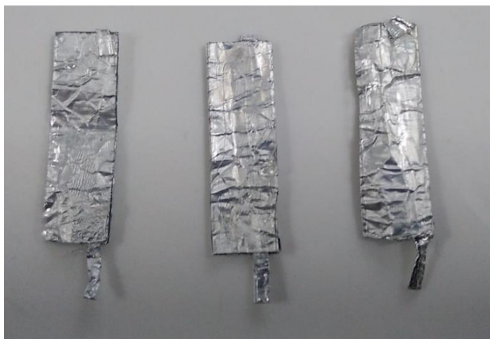
Figure 2.7. Bulk-NIP samplers, prepared by the dip-coating method.
