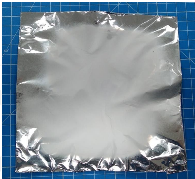
Figure 2.4. NIP polymer-coated aluminum foil
