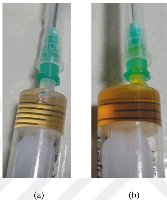
Figure 2.2. a) NIP and b) PMIP solutions prepared for electrospinning.
