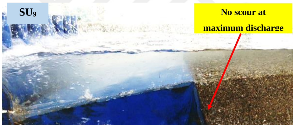
Figure 6.65 Scour region downstream the weir SU 9 .
