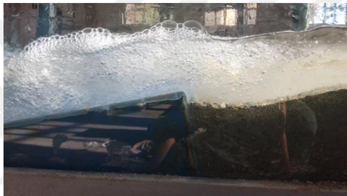
Figure 6.23 Scour depth behind the weir SU3 after 6 hours of experiment, Q = 0.02 \text{ m}^3\text{s}^{-1} .
