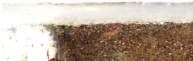
Figure 6.63 Scour depth behind the weir SU8 after 6 hours of experiment, Q = 0.02 \text{ m}^3\text{s}^{-1} .
