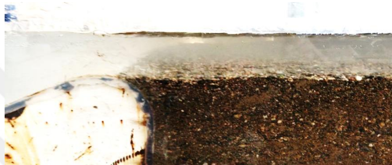
Figure 6.62 Scour depth behind the weir SU8 after 6 hours of experiment, Q = 0.015 \text{ m}^3\text{s}^{-1} .
