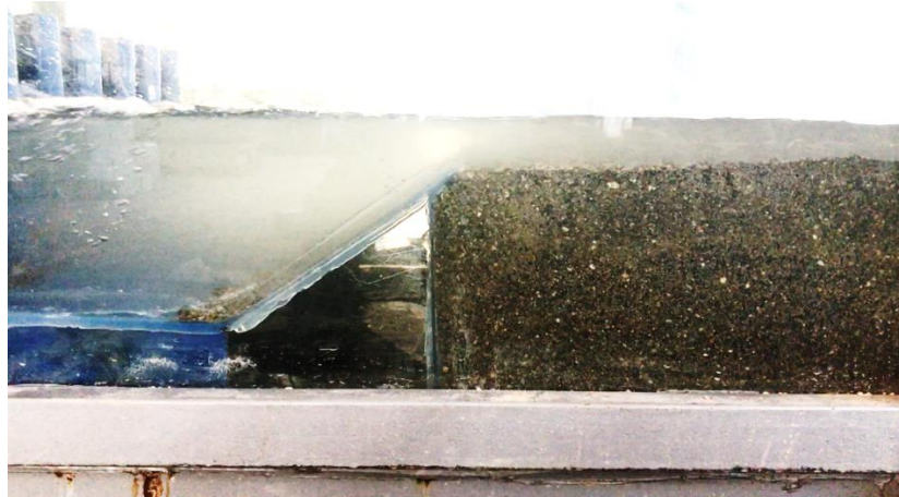
Figure 6.54 Scour depth behind the weir SU7 after 6 hours of experiment, Q = 0.015 \text{ m}^3\text{s}^{-1} .
