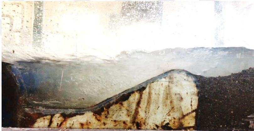
Figure 6.15 Scour depth behind the weir SU2 after 6 hours of experiment, Q = 0.02 m 3 s -1 .
