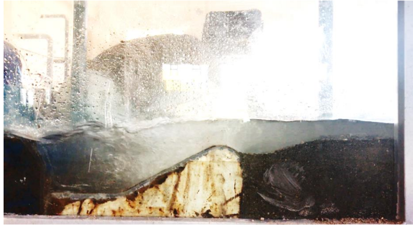
Figure 6.14 Scour depth behind the weir SU2 after 6 hours of experiment, Q = 0.015 m 3 s -1 .
