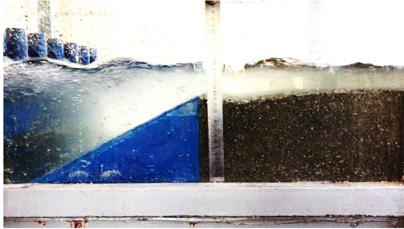
Figure 6.47 Scour depth behind the weir SU6 after 6 hours of experiment, Q = 0.02 \text{ m}^3\text{s}^{-1} .
