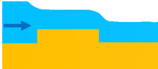
Figure 1.8 Flow over broad crested weir.
