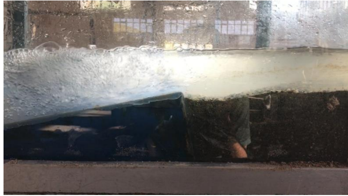
Figure 6.22 Scour depth behind the weir SU3 after 6 hours of experiment, Q = 0.015 \text{ m}^3\text{s}^{-1} .
