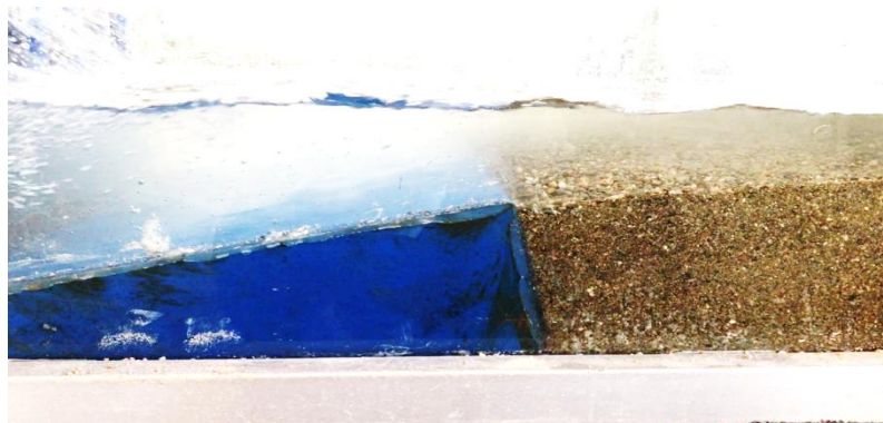
Figure 6.72 Scour depth behind the weir SU9 after 6 hours of experiment, Q = 0.025 \text{ m}^3\text{s}^{-1} .
