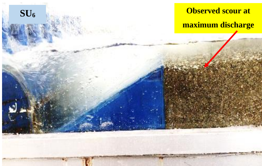
Figure 6.41 Scour region downstream the weir SU6.
