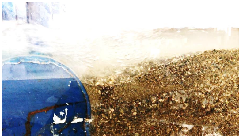
Figure 6.31 Scour depth behind the weir SU4 after 6 hours of experiment, Q = 0.02 \text{ m}^3\text{s}^{-1} .
