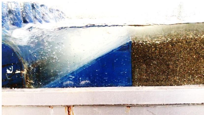
Figure 6.46 Scour depth behind the weir SU6 after 6 hours of experiment, Q = 0.015 \text{ m}^3\text{s}^{-1} .
