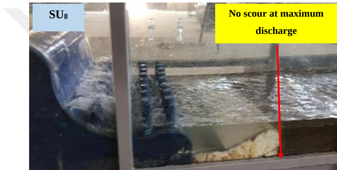
Figure 6.57 Scour region downstream the weir SU8.
