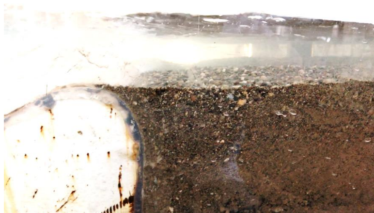
Figure 6.39 Scour depth behind the weir SU5 after 6 hours of experiment, Q = 0.02 \text{ m}^3\text{s}^{-1} .
