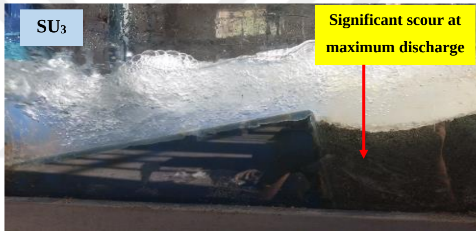
Figure 6.17 Scour region downstream the weir SU 3 .
