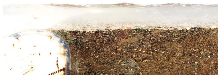
Figure 6.64 Scour depth behind the weir SU8 after 6 hours of experiment, Q = 0.02 \text{ m}^3\text{s}^{-1} .
