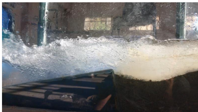
Figure 6.24 Scour depth behind the weir SU3 after 6 hours of experiment, Q = 0.025 \text{ m}^3\text{s}^{-1} .
