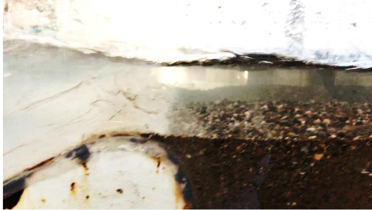
Figure 6.40 Scour depth behind the weir SU5 after 6 hours of experiment, Q = 0.02 \text{ m}^3\text{s}^{-1} .
