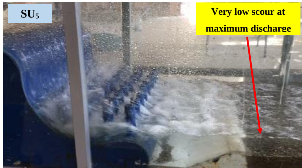
Figure 6.33 Scour region downstream the weir SU5.
