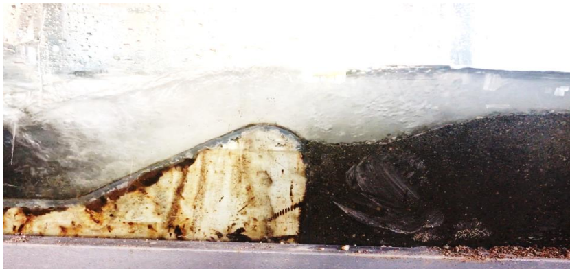
Figure 6.16 Scour depth behind the weir SU2 after 6 hours of experiment, Q = 0.025 m 3 s -1 .
