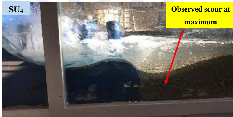
Figure 6.25 Scour region downstream the weir SU 4 .
