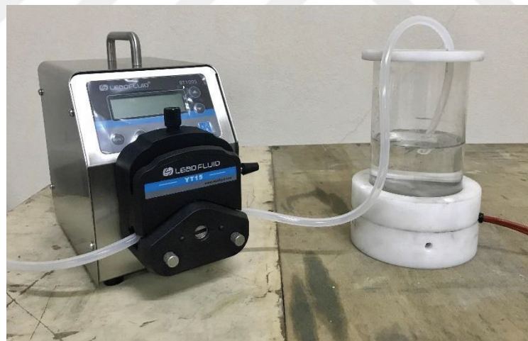
Figure 18: The Peristaltic Pump Used for The Liquid Circulation and The Manufactured Thermostat Assembly.
