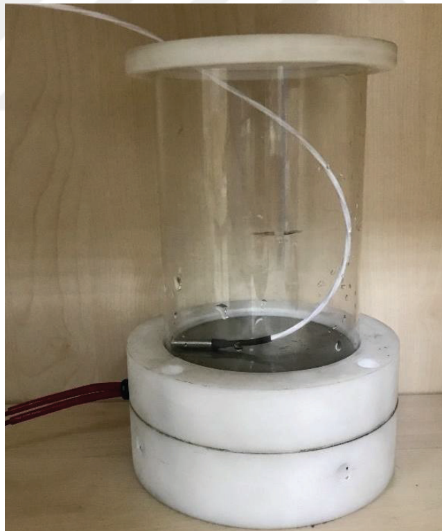
Figure 16: Manufactured Thermostat with Thermocouple Inside.
