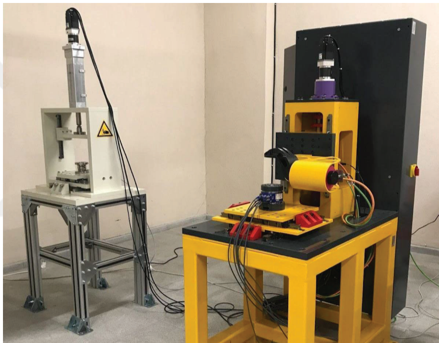
Figure 20: Physical Representation of The Manufactured Hip Joint Implant Wear Test Simulator and The Soaking Station.
