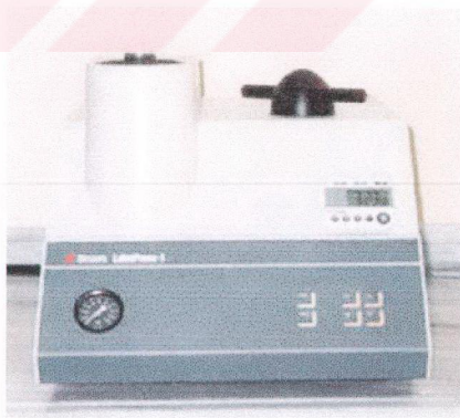
Figure 3.16. STUERS Labopress mounting test machine
