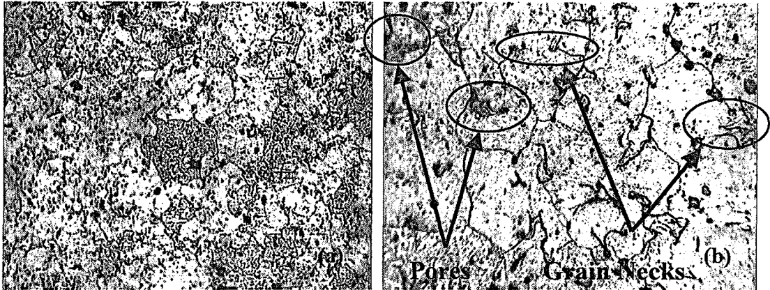
Figure 4.32. Fe 1200 °C, 30 min. Sintered Parts for 500 MPa (a-100X, b-400X)
