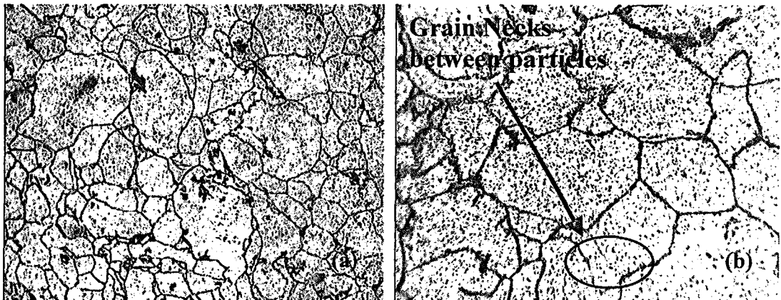
Figure 4.22. Al 20 min., 600 °C Sintered Parts for 600 MPa (a-100X, b-400X)
