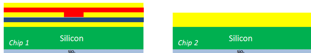
(e) Deposit 3 rd parylene layer
