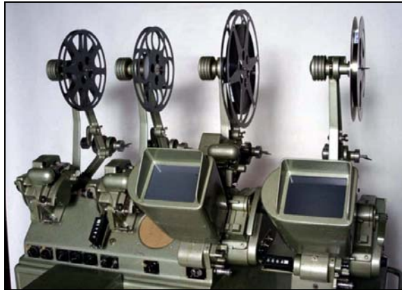
Figure 3.8 Moviola – The Machine that Workprint was Viewed and Cut. (Video University, 2011)
