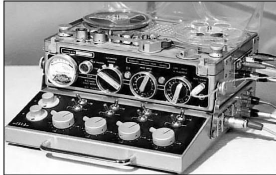
Figure 3.4 Earlier Sound Recording Equipment. (Academy Award winning NagraIII + Sela mixer recorder) (Nagra Recorder, 2011)
