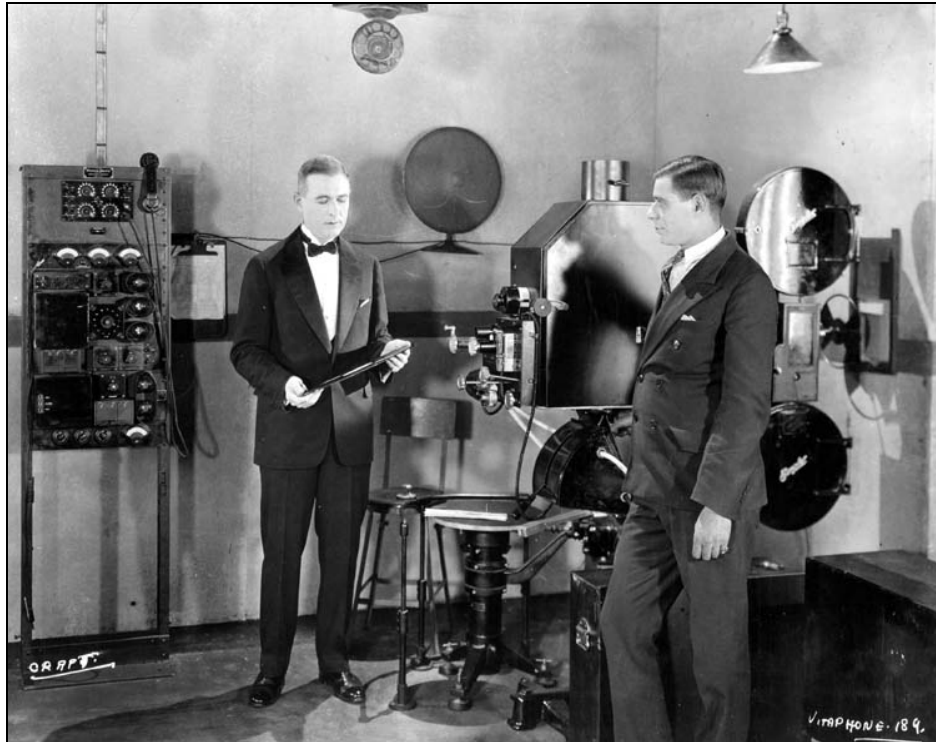
Figure 3.25 Vitaphone, Sound on Disk System (Wikipedia, 2011b)
