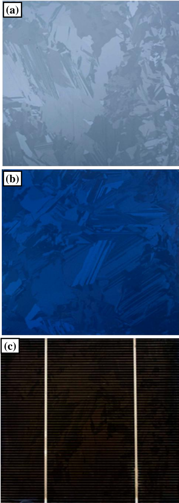
Figure 2.28. (a) Bare multicrystalline silicon (mc-Si) wafer, (b) mc-Si wafer with anti-reflective coating, (c) mc-Si solar cell with silicon nanowire arrays.
