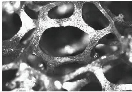
Figure 3.2 Closer view of open cell metal foam
