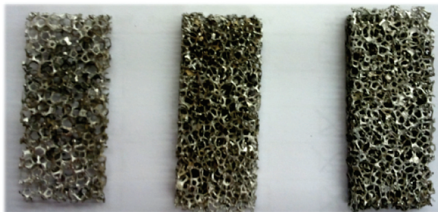
c. 40ppi metal foam pieces. Compression factor 1,2, and 3
