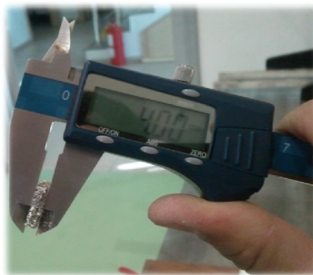
c. Final foam thickness
