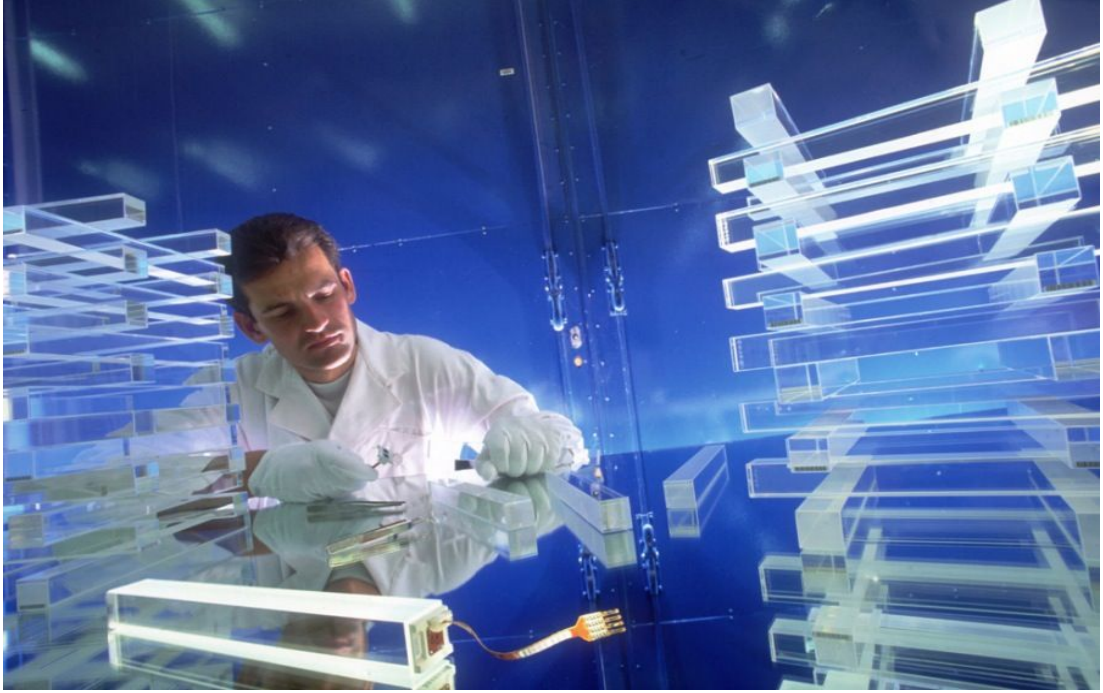
Şekil 2.6. Kurşun Tungstant Kristalleri ( http://cms.web.cern.ch/news/electromagnetic-calorimeter ).
