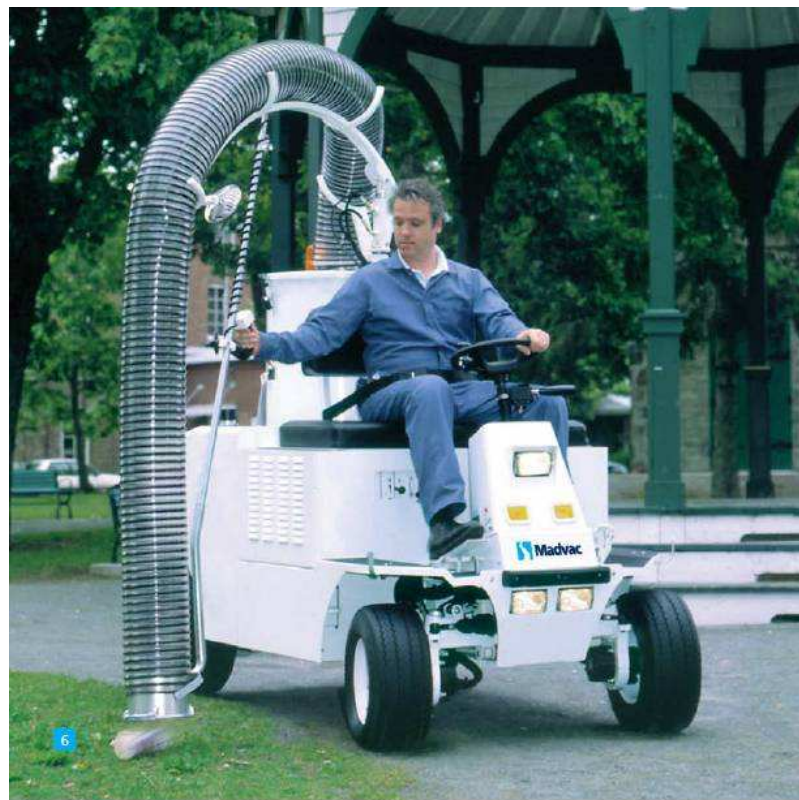
Figure 108 Elastic Vacuum Hose (MADVAC 101)
