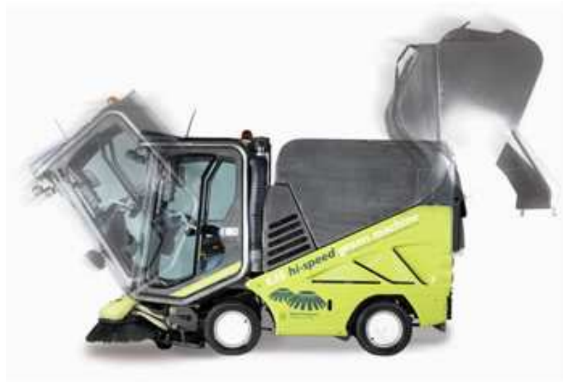
Figure 14 Green Machine 636HS during discharging [13]
