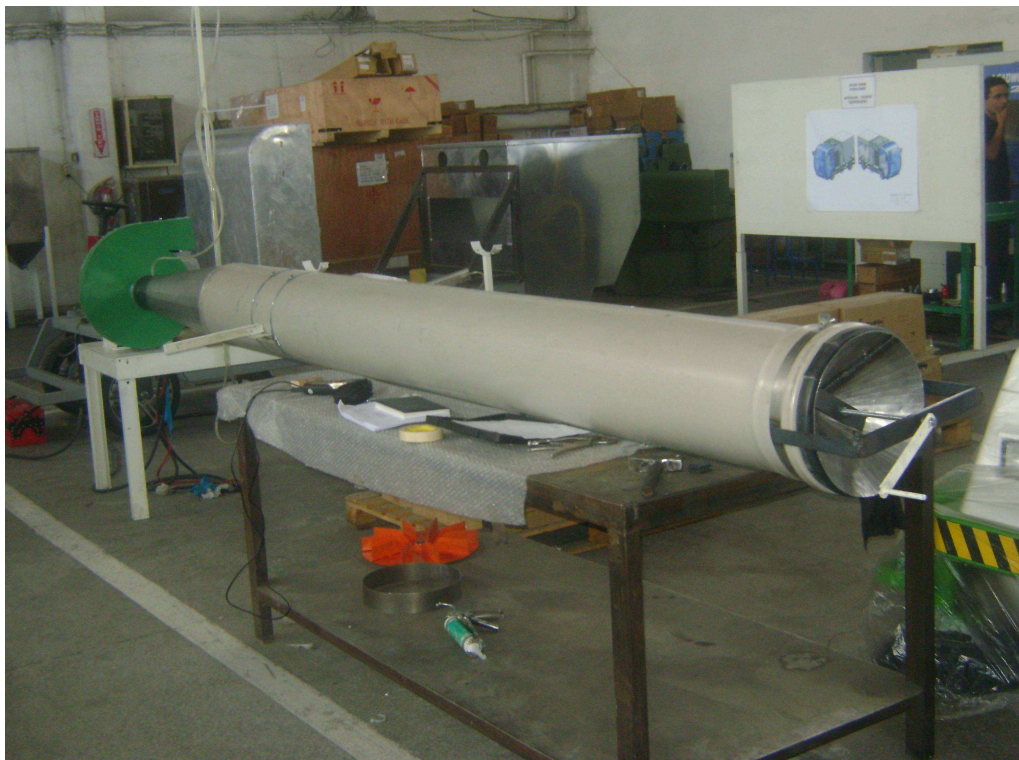
Figure 74 Test Setup for New Fans
