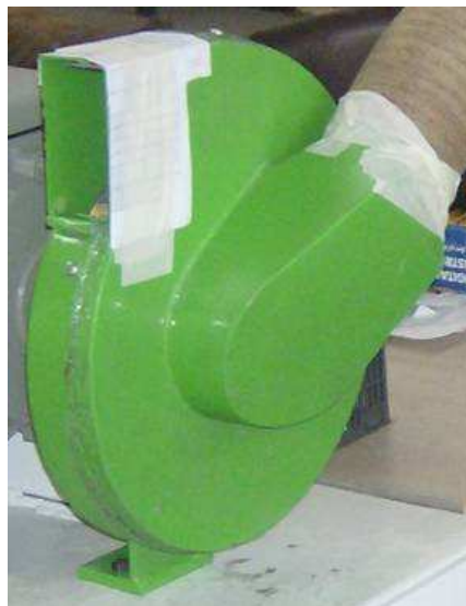
Figure 40 Former Müsan Fan (D= 250 mm)
