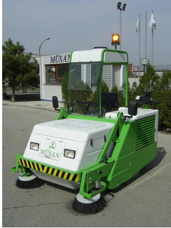
Figure 3 Müsan VSM 060 Sweeper [6]
