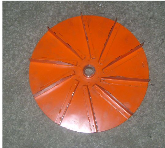
Figure 43 Welding of Blades around the Fan Rotor (D=400 mm & 10 Blades)
