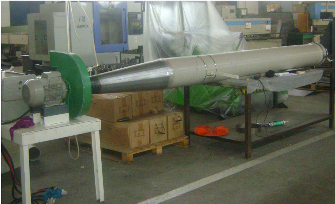
Figure 64 Test Setup for the New Fans
