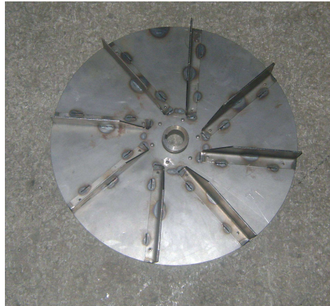
Figure 42 Welding of Blades around the Fan Rotor (D=400 mm & 8 Blades)
