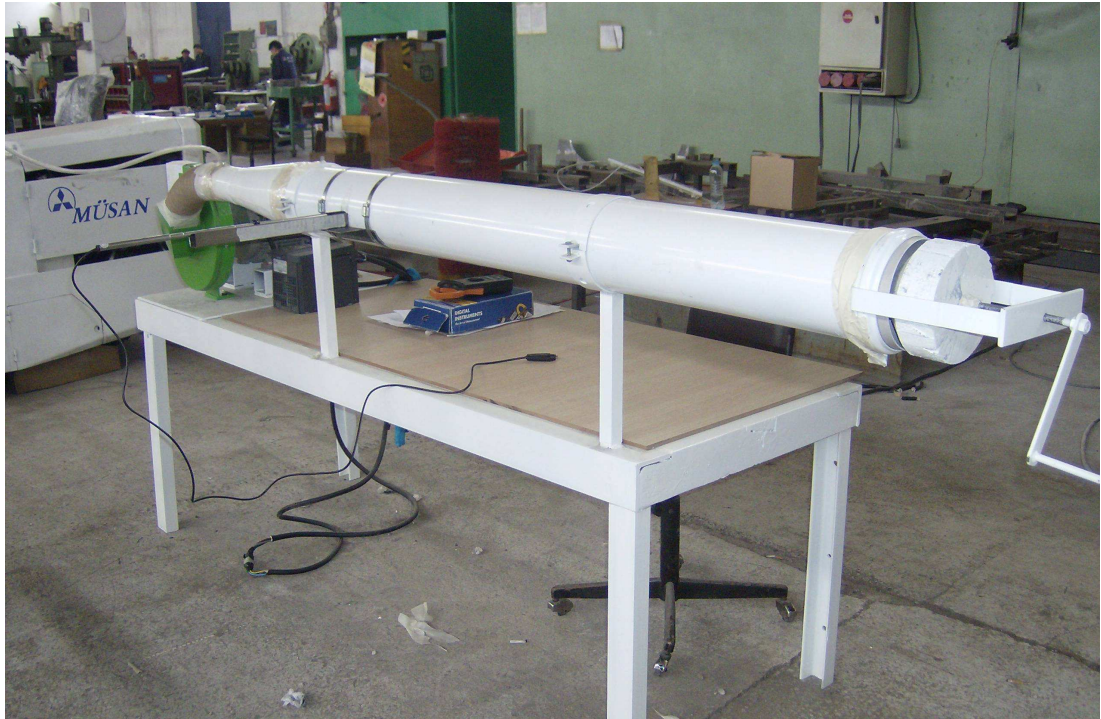
Figure 60 Test Set-Up for the Experiments of Current Fans
