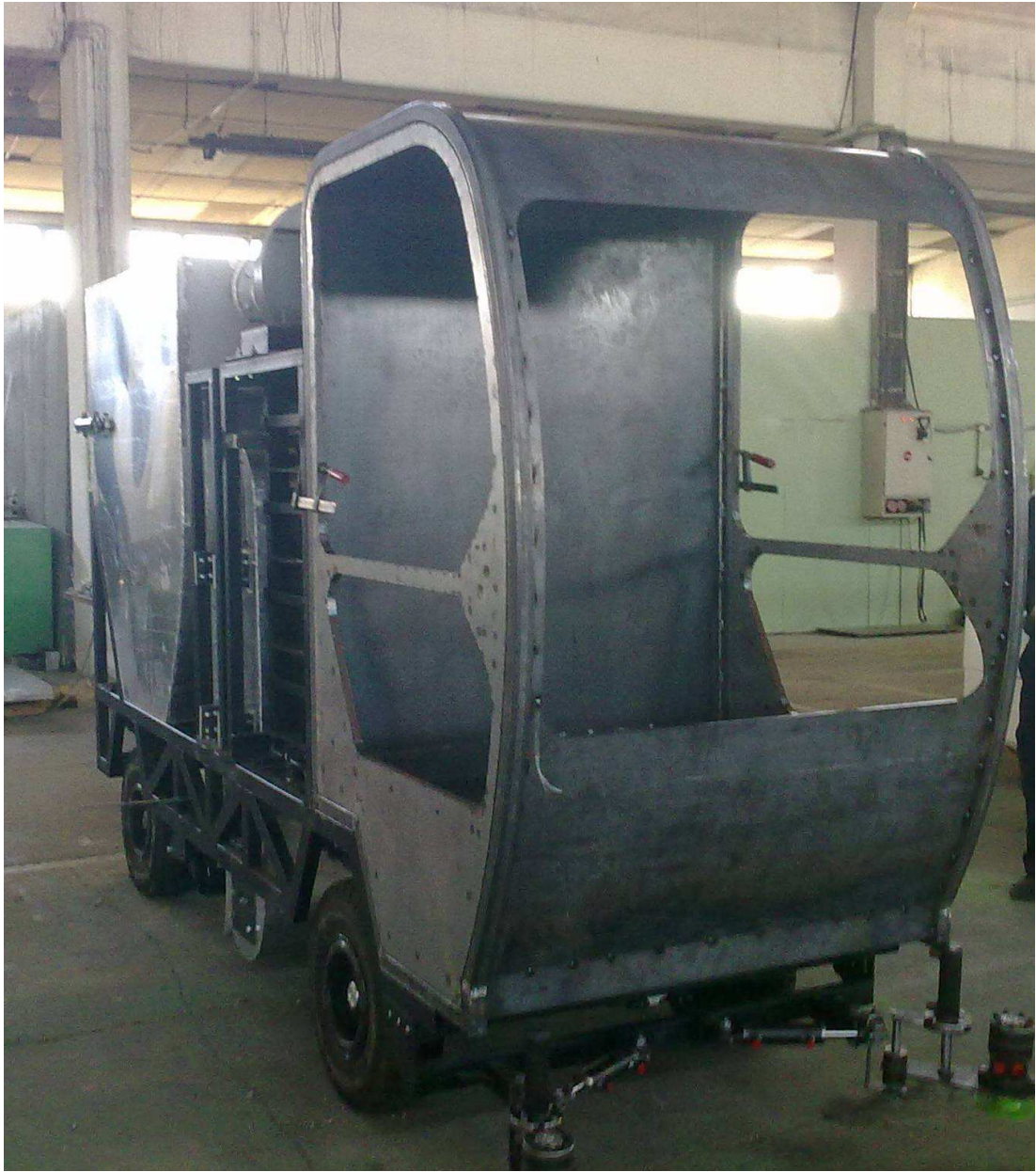
Figure 120 VSM 080 Sweeper before the External Cladding and Accessories
