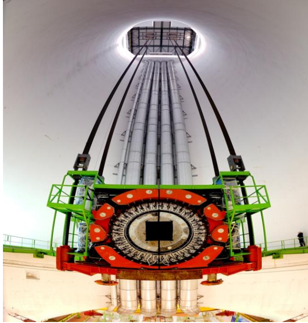
Şekil 3.14. Hadronik İleri Klorimetre ( http://cds.cern.ch/record/1431489/files/HFLowering4.jpg?subformat=icon-1440 ).
