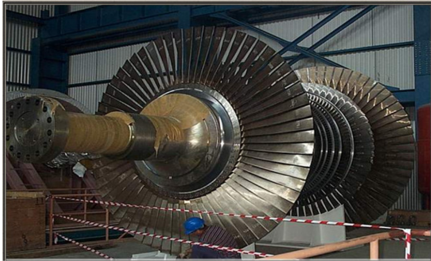
Figure 3.5. LP turbine moving blades
