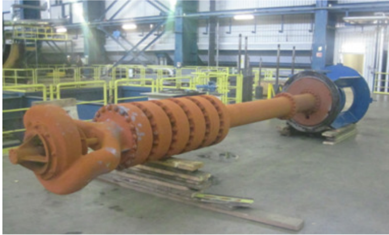
Figure 3.9. Condenser extraction pump
