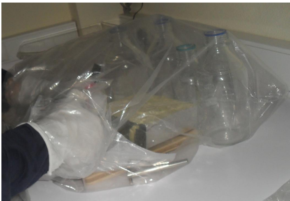
Figure III. 9 Core foam sampling in glove bag
