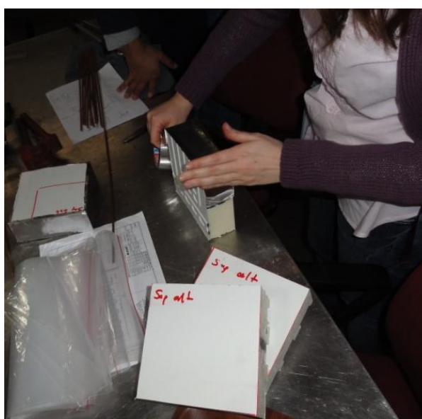
Figure III. 4 Wrapping of samples with aluminum tape
