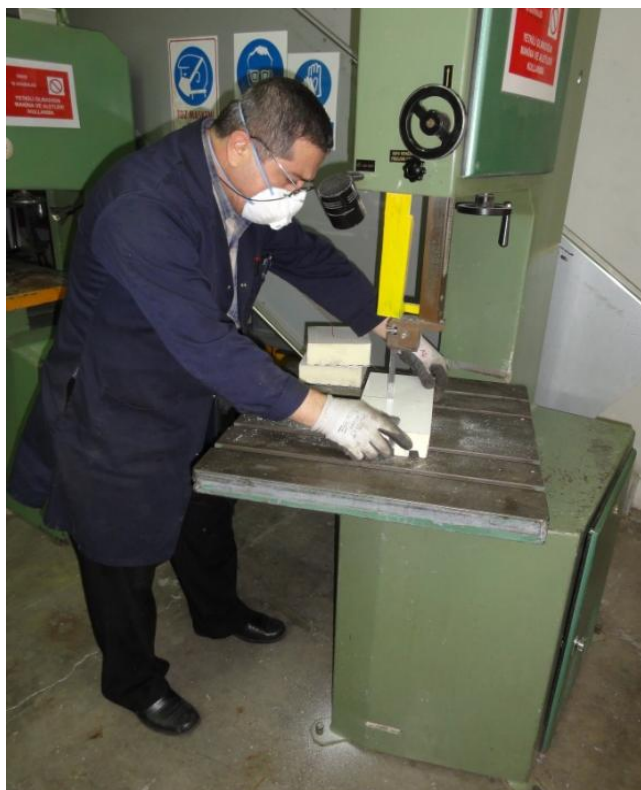
Figure III. 3 Cutting of foam panels into desired sizes (15×15 cm) after removal from the unit
