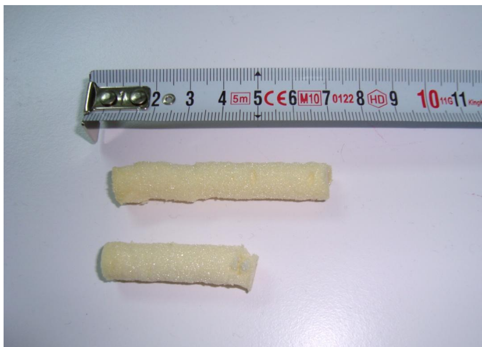
Figure IV. 8 Foam samples from freezer and fridge
