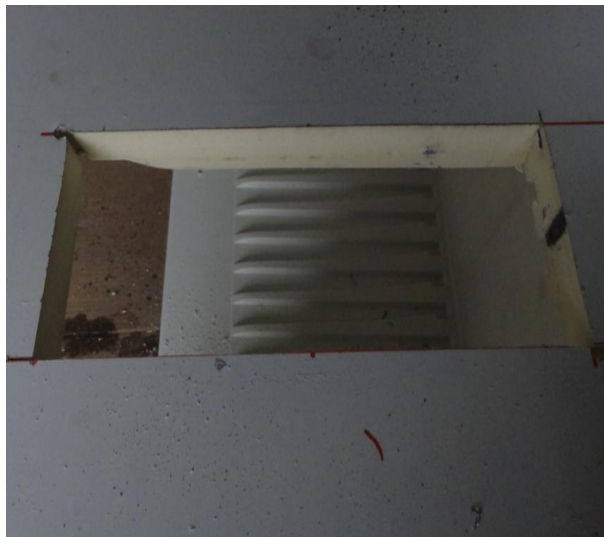
Figure III. 2 Foam sampling from refrigerator
