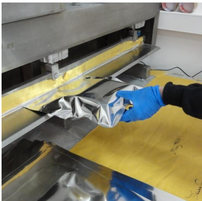
Figure III. 5 Placing foam panels in Tedlar bags
