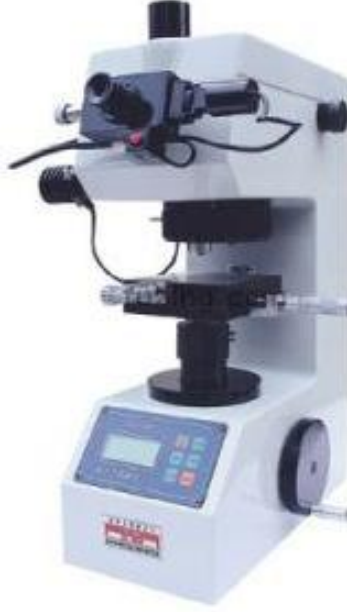
řekil 3.19. HVS-1000 Digital Display Microhardness Tester model test cihazı
