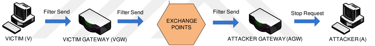
Figure 2.5. Active Internet Traffic Filtering (AITF) [5]. Filter is sent from victim (V) to its gateway (VGW). Then it is propagated to the attacker's gateway (AGW) which requests attacker (A) to stop sending traffic.
