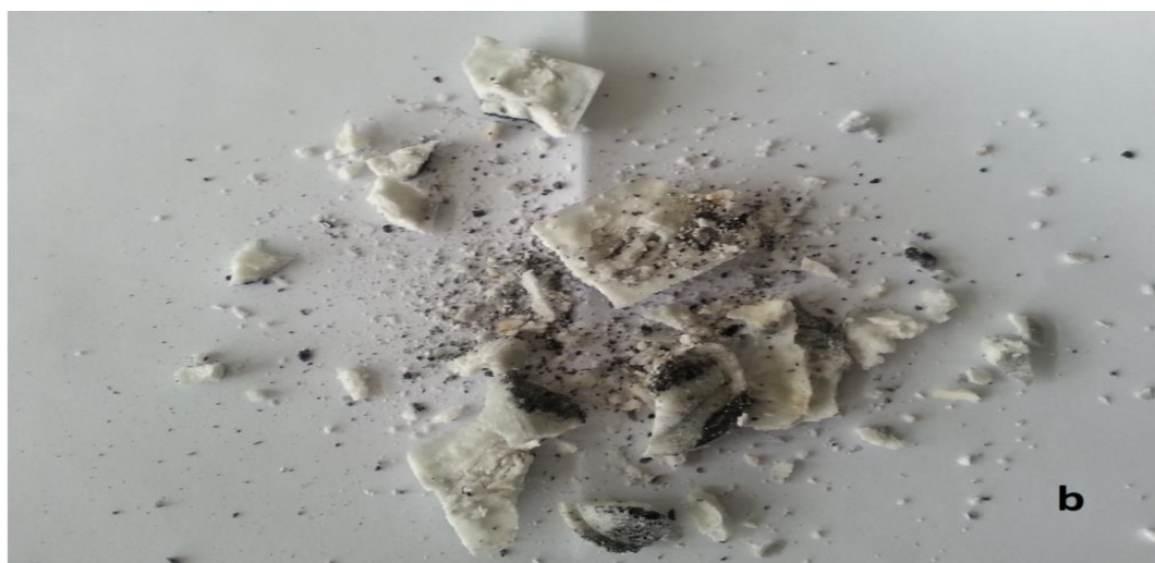
Figure 5.1 FTIR spectra's of the waxy product (a). product picture (b). (catalyst: Pd/C, temperature: 375 °C, initial H 2 pressure: 3 MPa, reaction time: 60 min.)
