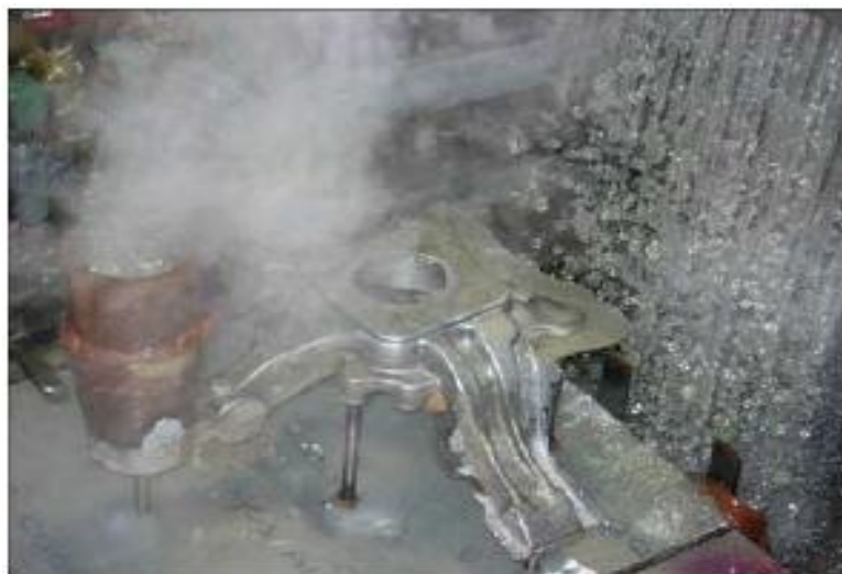
Figure 1.42 Completion of ablation casting[34]
