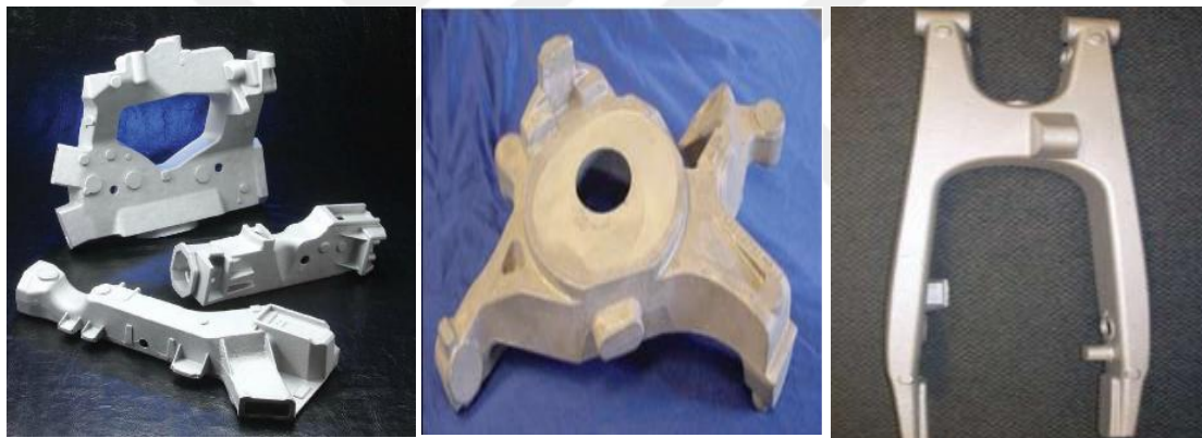
Figure 1.44 Ablation cast a) joints[38] b) steering knuckle c) B206 alloy swing arm[34]
