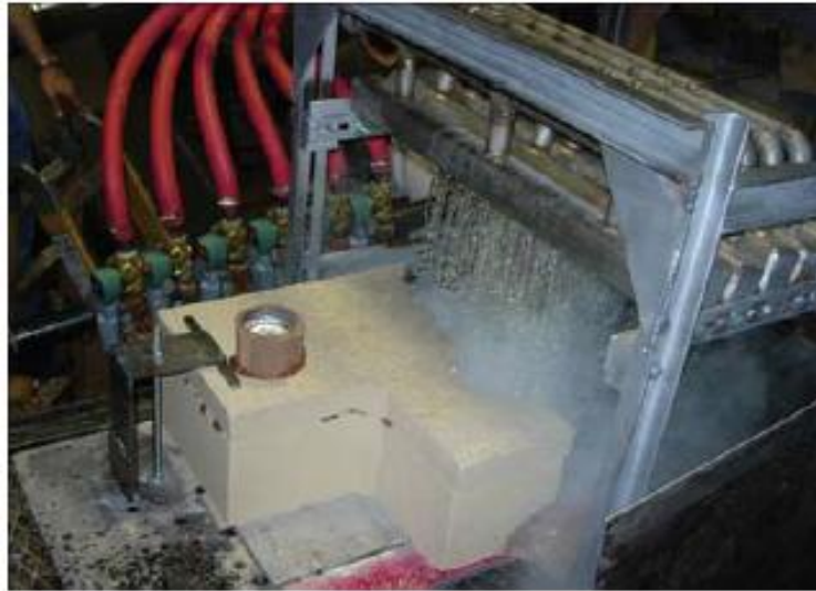
Figure 1.41 Ablation of aggregate sand mold by a water jet[34]
