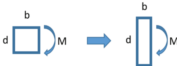
Figure 4.4. Cross sections transformation in Model 3
