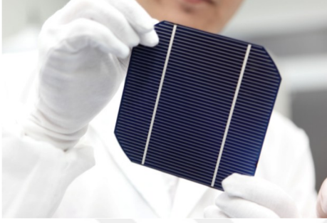
Resim 4.1. Mono kristal PV panel
