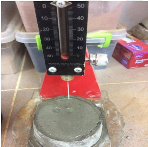
Figure 3.15 The Vicat apparatus that used in this study during the test process
