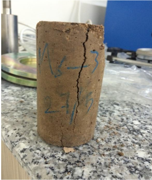
Figure 3.10 Sample after failure
