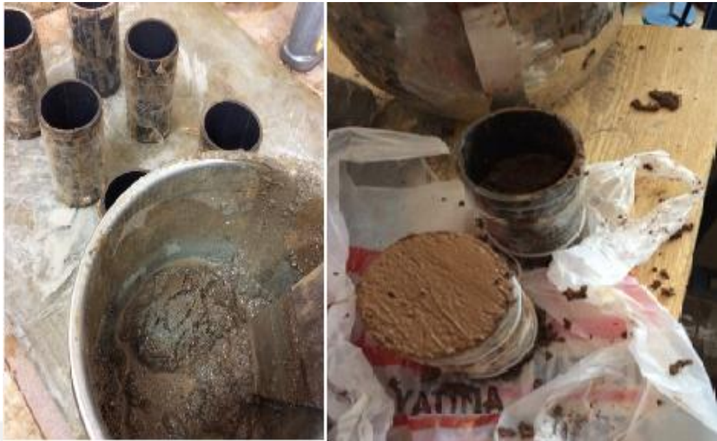
Figure 3.5 Plastic moulds used and sample preparation
