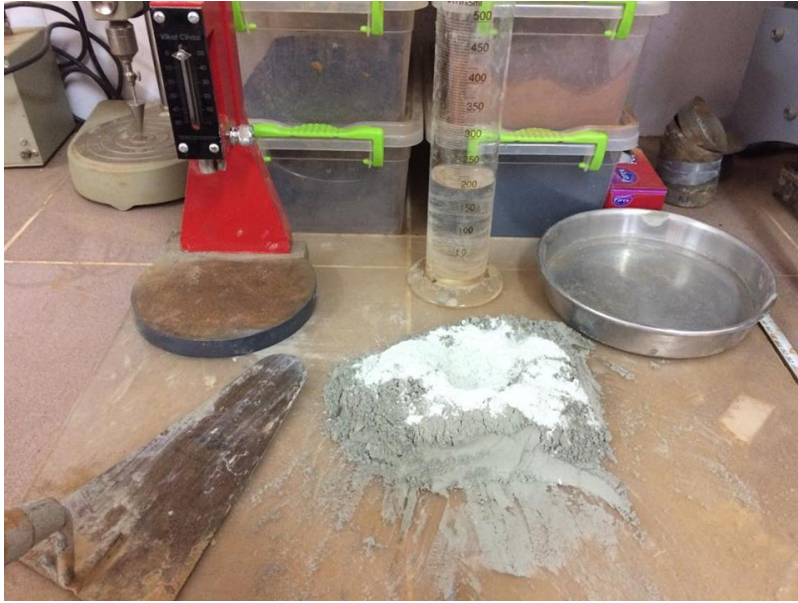
Figure 3.14 Appeared the preparation of cement mixed with soda waste glass powder for Vicat test
