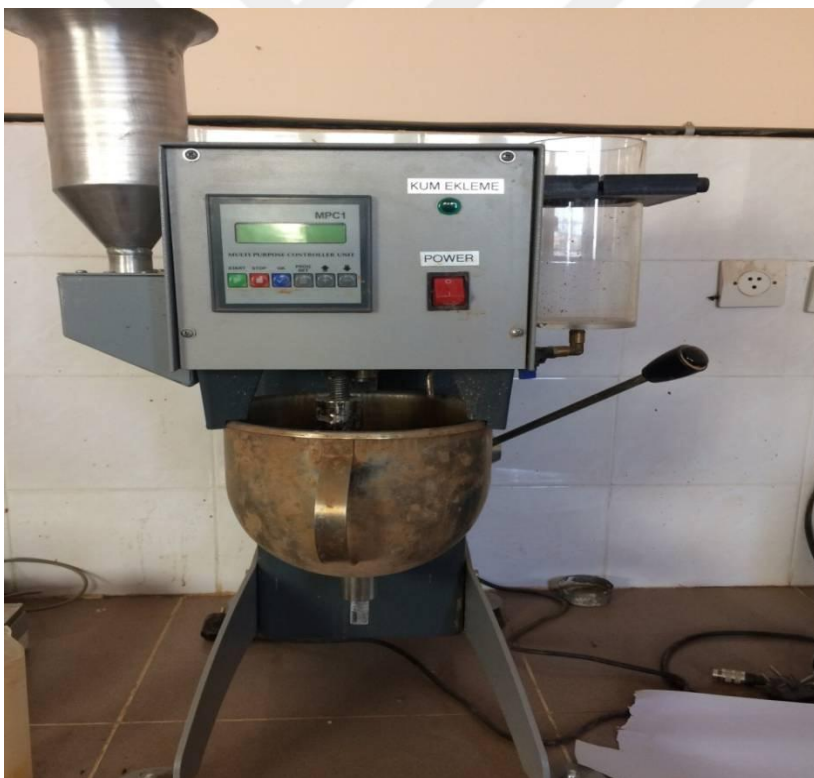
Figure 3.4 Electrical mixer that used to mix the ingredients in this study
