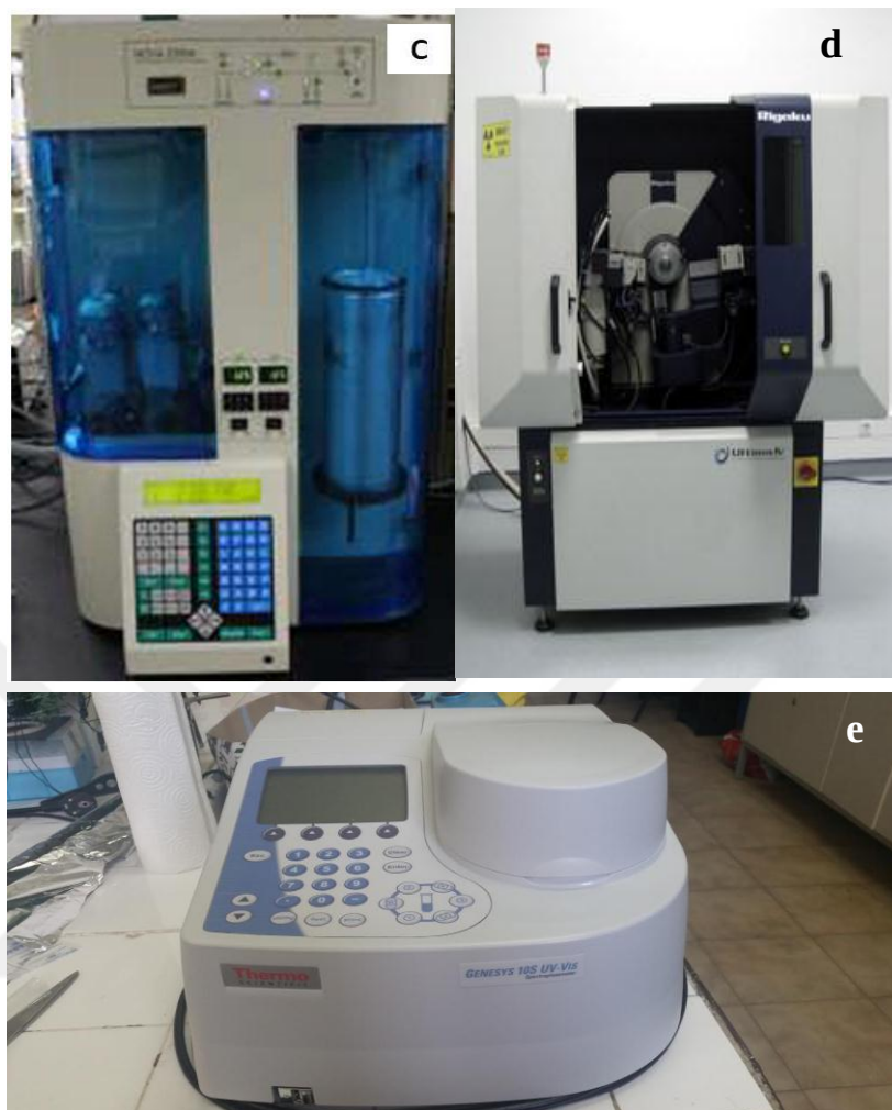
Figure 3.1. The equipment used for the characterization of bare chitosan microgel beads, bare \text{TiO}_2 spheres, gold nanoparticles and heterogeneous catalysts a) QUANTA 400F Field Emission SEM-EDAX b) CTEM, FEI Tecnai G2 Spirit BioTwin c) Surface Area and Pore Size Analyzer, Quantachrome Nova 2200 d) XRD, Rigaku Ultima IV e) UV-Vis Spectrophotometer, GENESYS 10S, Thermo Scientific
