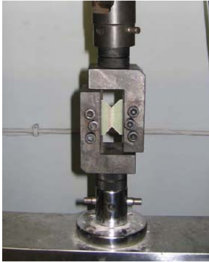
Figure 4.11 V-notched rail shear test process
