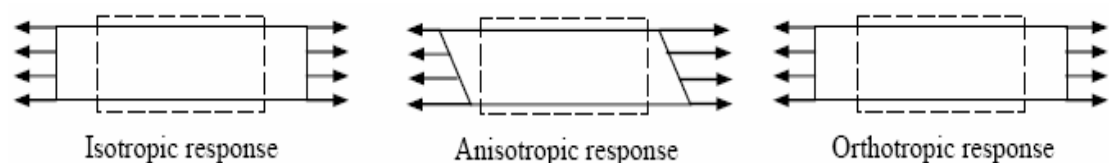
Figure 2.2 Typical material response for isotropic, anisotropic, and orthotropic materials subjected to axial tension
