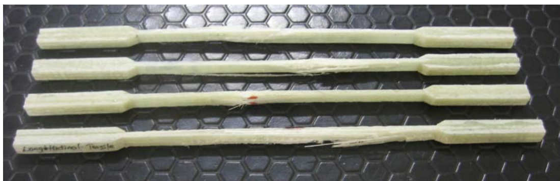
Figure 4.3 Deformed tensile test specimens to obtain longitudinal elasticity module ( E_1 ) and poisson ratio ( \nu_{12} )
