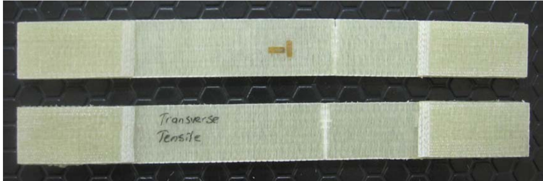
Figure 4.5 Deformed tensile test Specimens to obtain transverse elasticity module ( E_2 ) and poisson ratio ( \nu_{21} )
