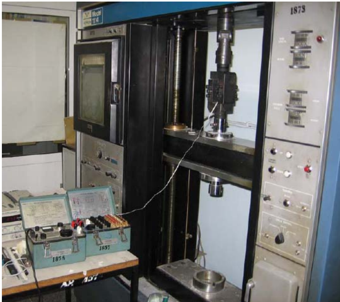
Figure 4.13 Connected indicators to the specimen in V-notched rail shear test process
