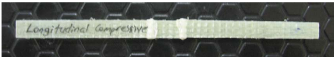
Figure 4.7 Deformed longitudinal compressive test specimens to obtain longitudinal compressive strength ( X_c )
