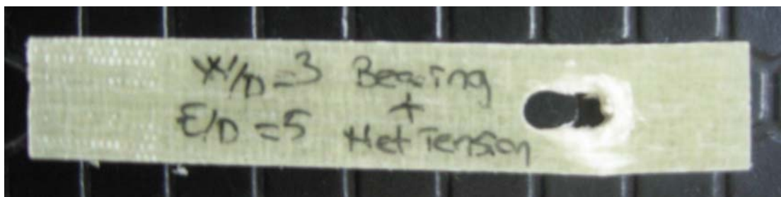
Figure 6.9 The photograph of tested specimen where occurred bearing and net tension together. (3 month sea water immersed)
