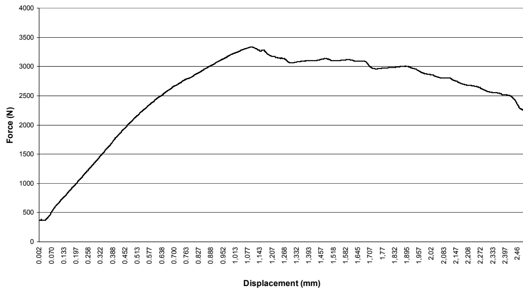
Figure 6.11 The characteristic of shear-out failure mode curve of a specimen ( 9 month sea water immersed, W/D=3 and E/D=2 )
