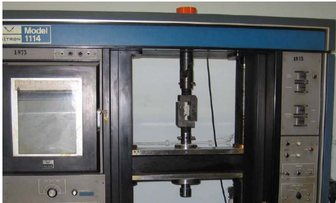
Figure 4.1 A view of the Instron 1114 test machine
