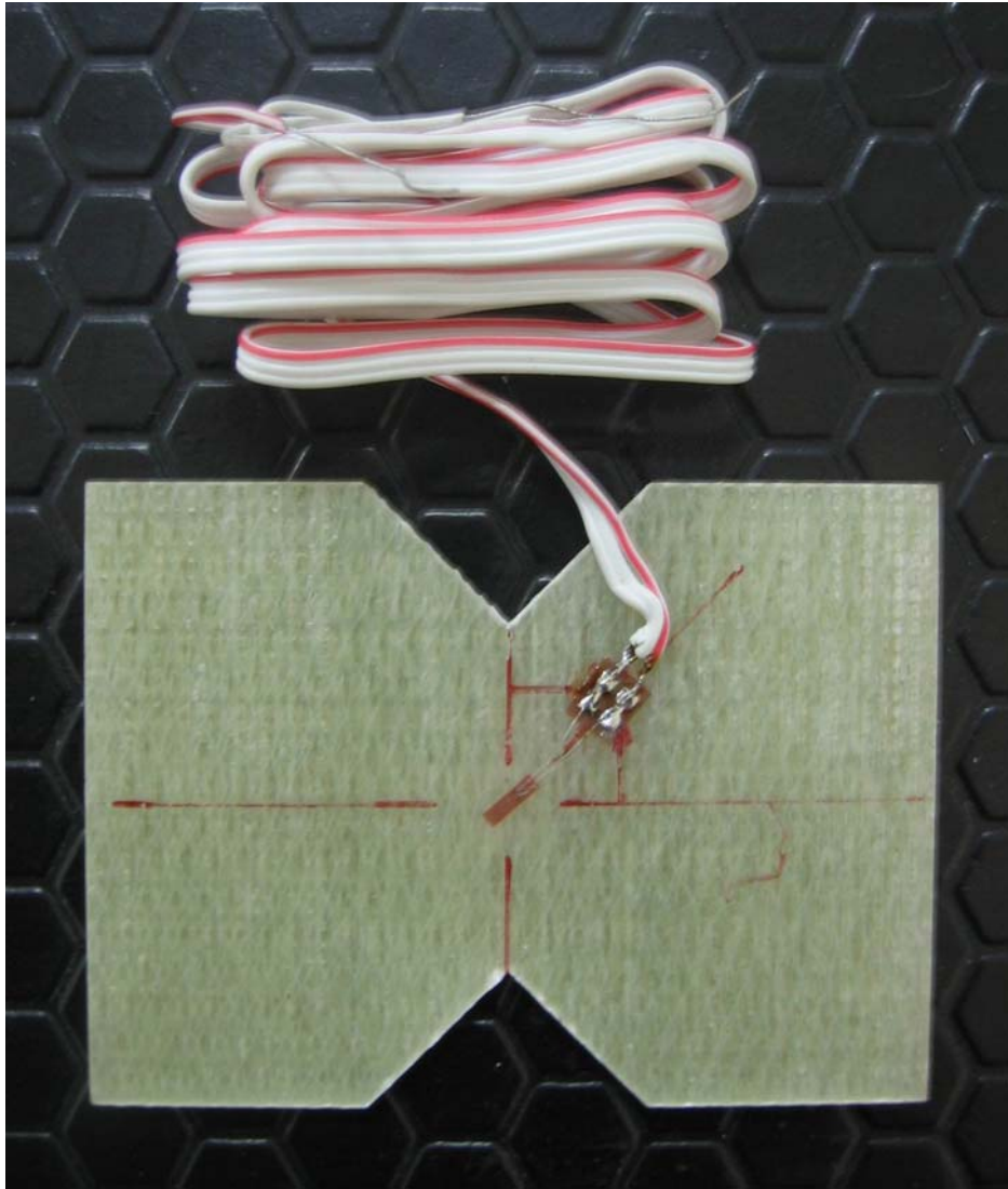
Figure 4.10 V-notched rail shear test specimen before tested.
