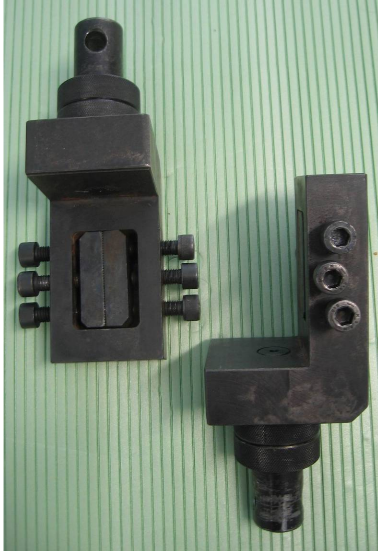
Figure 4.9 V-notched rail shear test equipment
