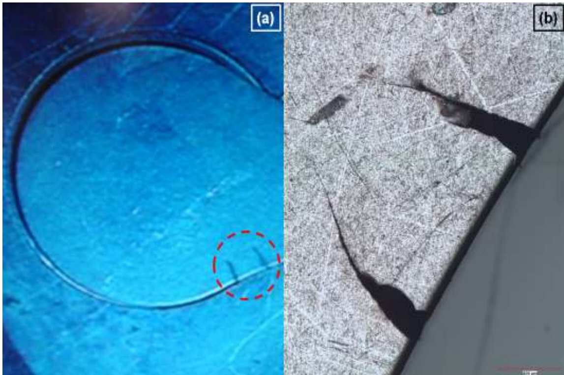
Figure 4.48. Valve leaf double crack origin (a) stroboscopic image of top face and (b) microscopic display of impact face
