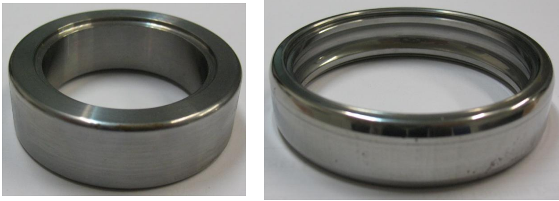
Figure 5 Final ring workpiece (right) rolled from the blank ring (left)
