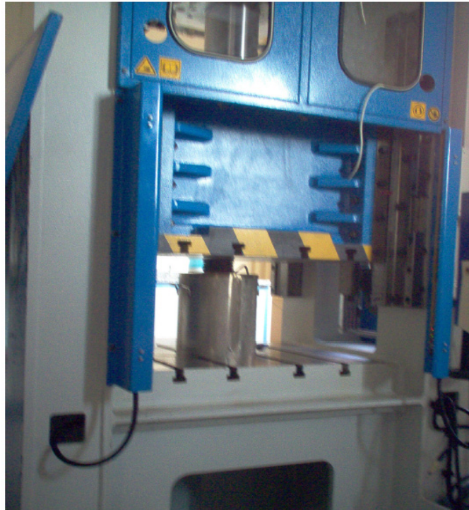
Figure 5.5 Squeeze casting mechanism and hydraulic press.
