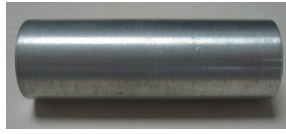
Figure 3.3. Specimen used in compression testing
