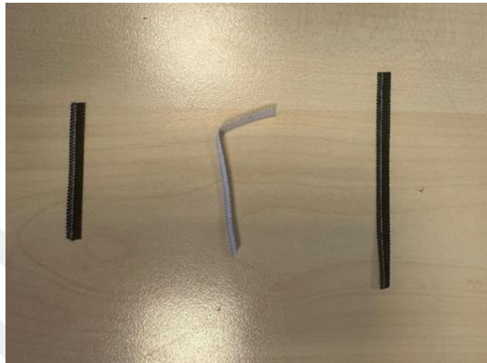
Figure 3.8. Examples of RFID Tags Deformed Due to Sewing Defects and an Intact Tag
