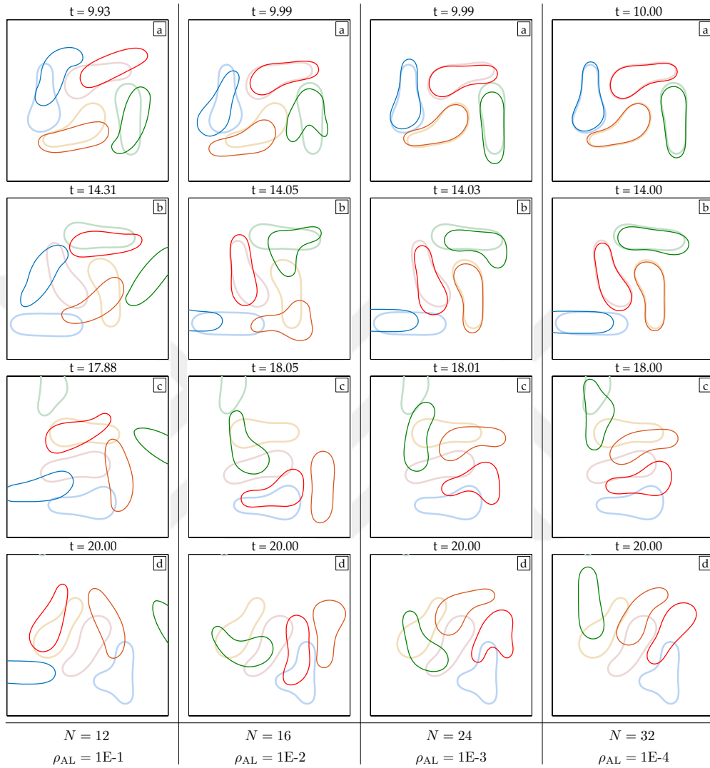
Figure 2.18: Four vesicles in the Taylor-Green flow with no viscosity contrast and with the LRCA. The spatial resolutions and the error tolerances are given at the bottom of each column. Faded vesicles correspond to the ground truth and the low-resolution counterparts are in bright colors.
