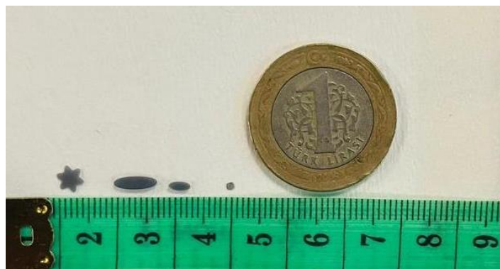
Figure 29 Fabricated Magnetic Swimmers, Size Comparison with the Coin
