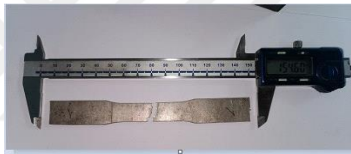
Figure 5.4. Tensile test measurement after the test.
