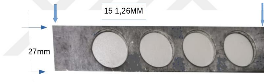
Figure 5.14. Dimensions of punch geometry (length 151.26mm, width 27mm).
