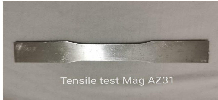
Figure 4.3. Tensile test samples of Mg AZ31 alloy.
