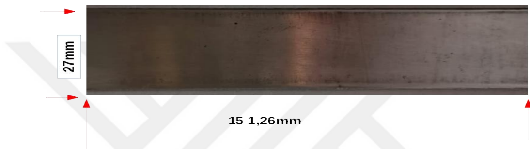
Figure 4.11. Dimensions: Thickness 3mm, length 151.26mm, and width 27 mm.
