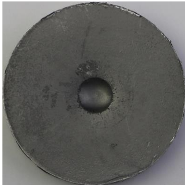
Figure 5.3. The after-impact front and rear face views of the Al6061 plate.
