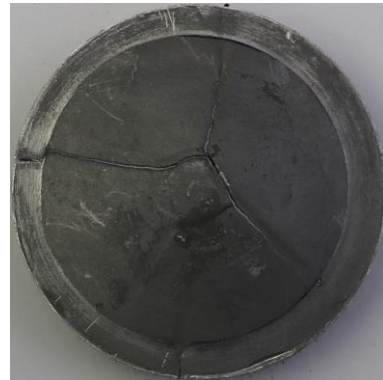
Figure 5.6. The after-impact front and rear face views of the ceramic-rich FGM plate.
