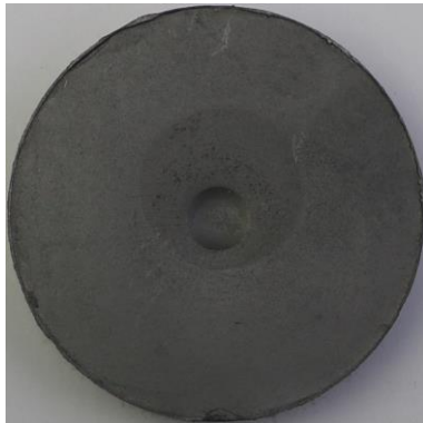
Figure 5.5. The after-impact front and rear face views of the linear FGM plate.
