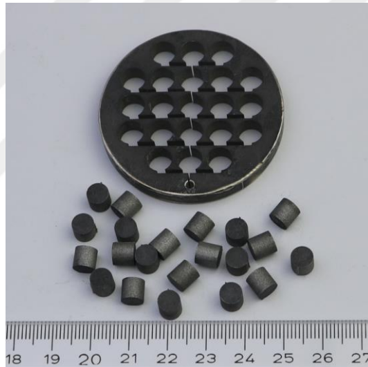
Figure 2.7. A group of compression test specimens prepared by the EDM.
