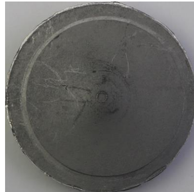
Figure 5.3. The after-impact front and rear face views of the Al6061 plate.
