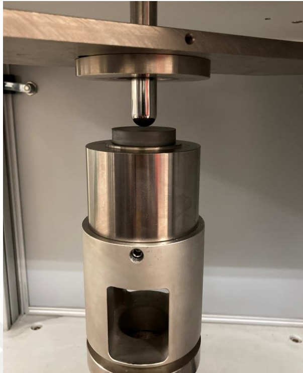
Figure 5.2. The boundary conditions of the low-velocity impact tests.
