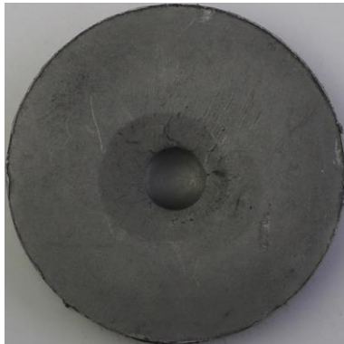
Figure 5.4. The after-impact front and rear face views of the metal-rich FGM plate.
