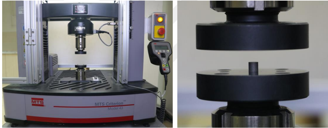
Figure 4.1. The testing machine and a quasi-static compression test setup.
