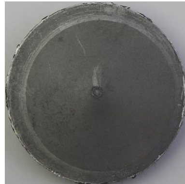
Figure 5.4. The after-impact front and rear face views of the metal-rich FGM plate.
