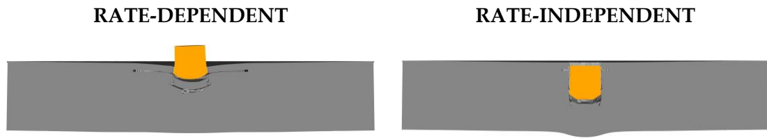
Figure 6.28. The effect of strain-rate dependency of the 50%SiC and 60%SiC layers on the numerical results for the linear FGM plate (500 m/s).
