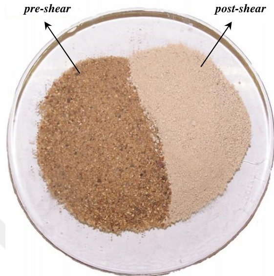
Figure 2.35. Specimens before and after ring shear test (from the shear band) (Sadrekarimi and Olson, 2010)
