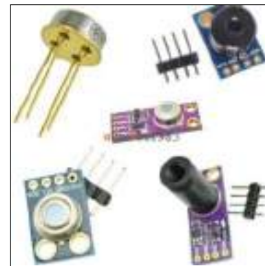
Figure 63: MLX90614 Non-contact Infrared Thermometer / Sensor (Melexis, 2013)
