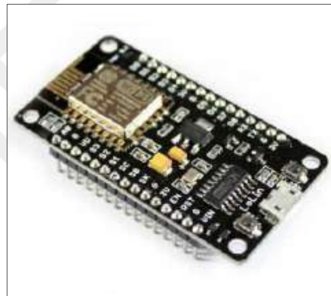
Figure 117: NodeMCU Board (NodeMCU, 2014)
