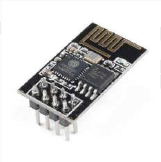
Figure 99: ESP8266 Wi-Fi Module (Sparkfun, 2015)
