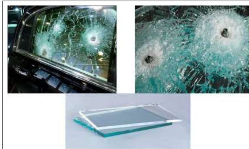
Figure 3.2. Polycarbonate backed silicon oxide bulletproof glass [24].
