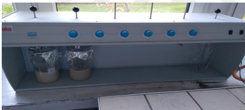
Figure 18. Equipment ENVAG stir equipment Flocculation Tester FC65
