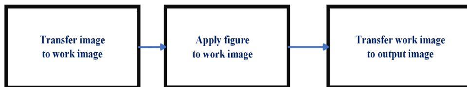
Figure 4.6. The vision sensor with three components.
