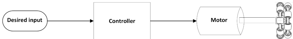
Figure 3.3. Open-loop control system.
