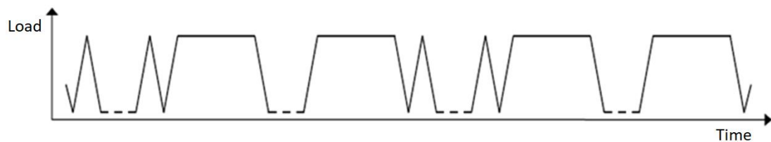
Figure 4.6 : Schematically expression of Block test [44].
