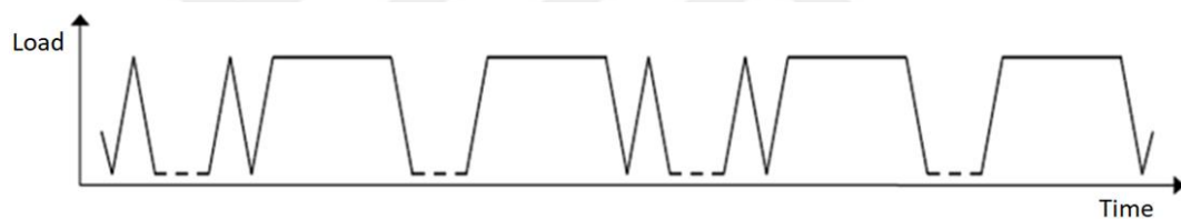
Figure 6.6 : Schematically expression of Block test [44].
