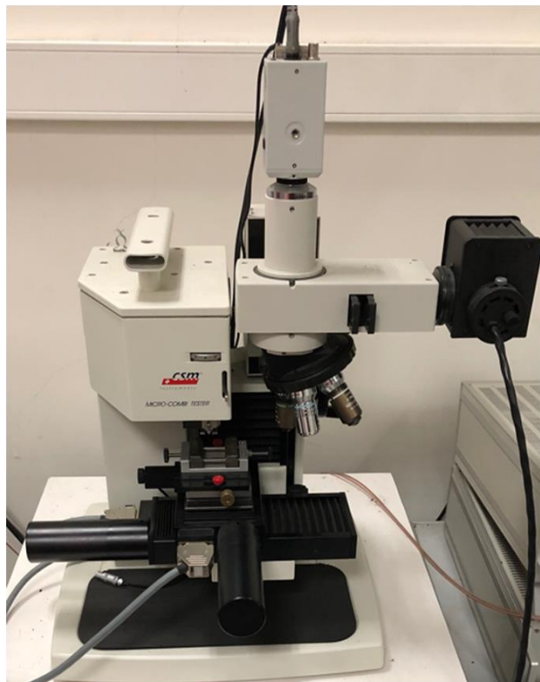
Figure 5.7 : CSM Micro-Combi tester nano indentation testing machine.
