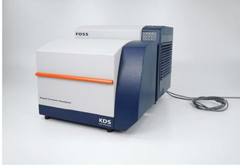
Şekil 11. Foss NIRSystem XDS Near-Infrared Rapid Content Analyser
