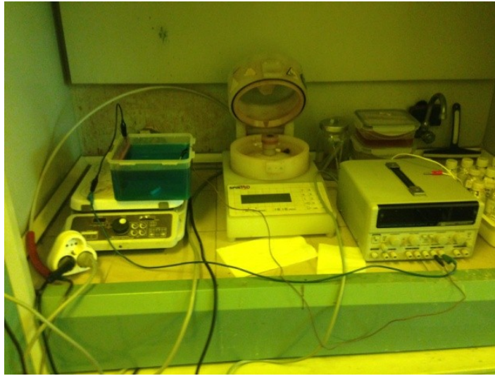
Figure 4.32 Copper electroplating setup.
