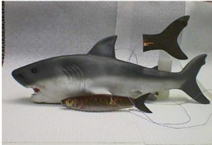
Figure 1.8 A designed and fabricated undulating caudal fin actuator and two robotic fish equipped with IPMC fin actuator (Shahinpoor & Kim, 2005)
