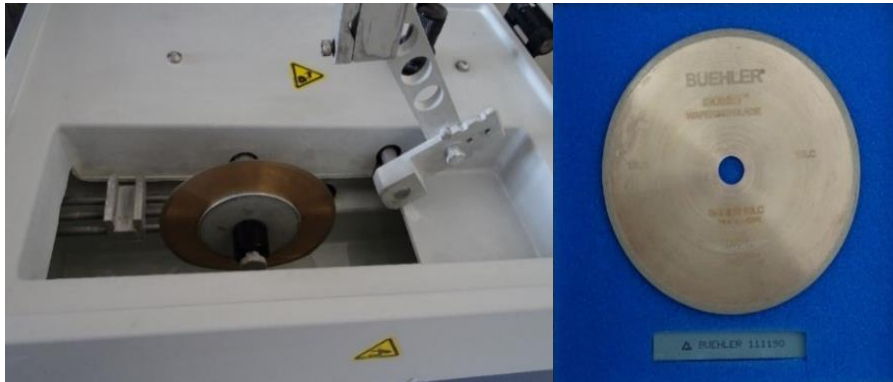
Resim 3.3. Elmas kesici disk (15LC, 11-4255, 127x0,4mm)
