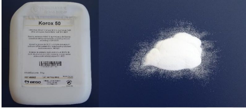
Resim 3.45. 50 \mu\text{m} \text{Al}_2\text{O}_3 kumu
