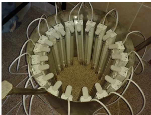
Figure 5.1 UV reactor for photocatalytic treatment
