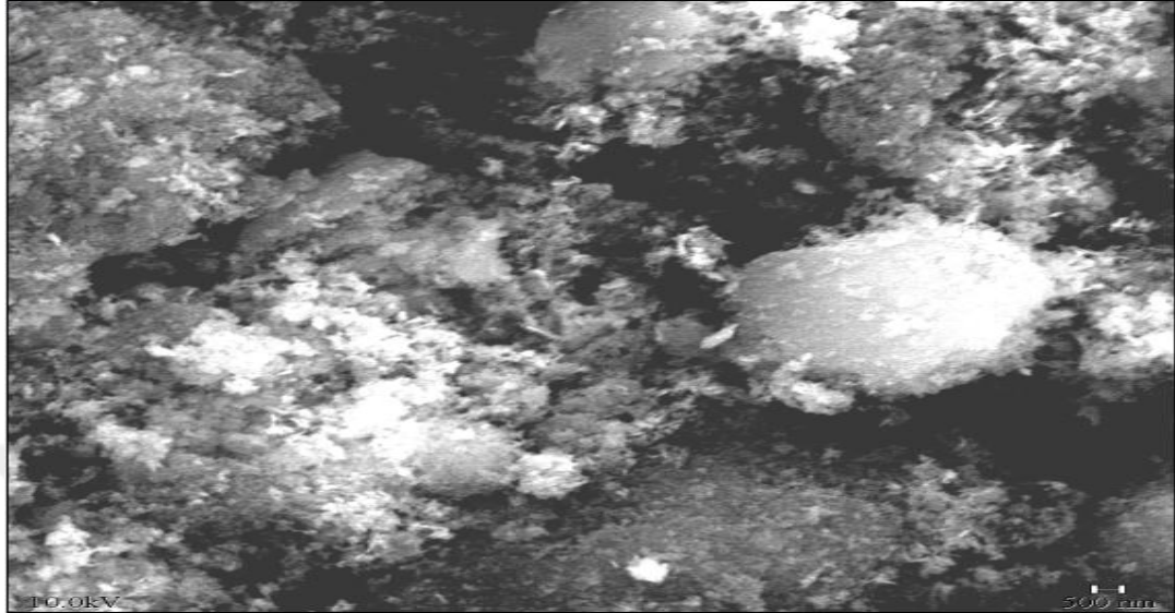
Figure 6.9 SEM image of raw nano-ZnO-SiO 2 composite (the molar ratio of ZnO:SiO 2 1:1)
