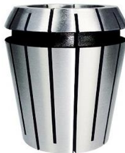
Figure 4.4 ER32 collet used in SRCS
