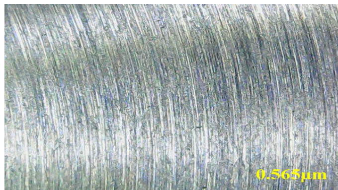
Figure 5.12 Machined surface images of AA5083 material (x25) d=0.5mm (a) Operator A (b) Operator B (c) SRCS
