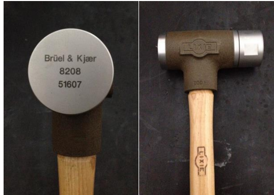
Figure 3.8 Impact hammer for natural frequency measurement used for experimental studies
