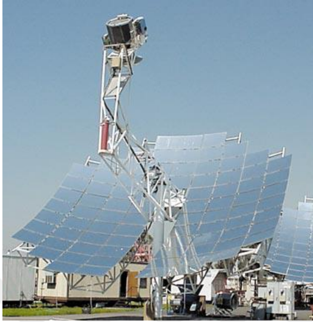
Figure 3. Boing/SES DECC Dish Stirling System[2]
