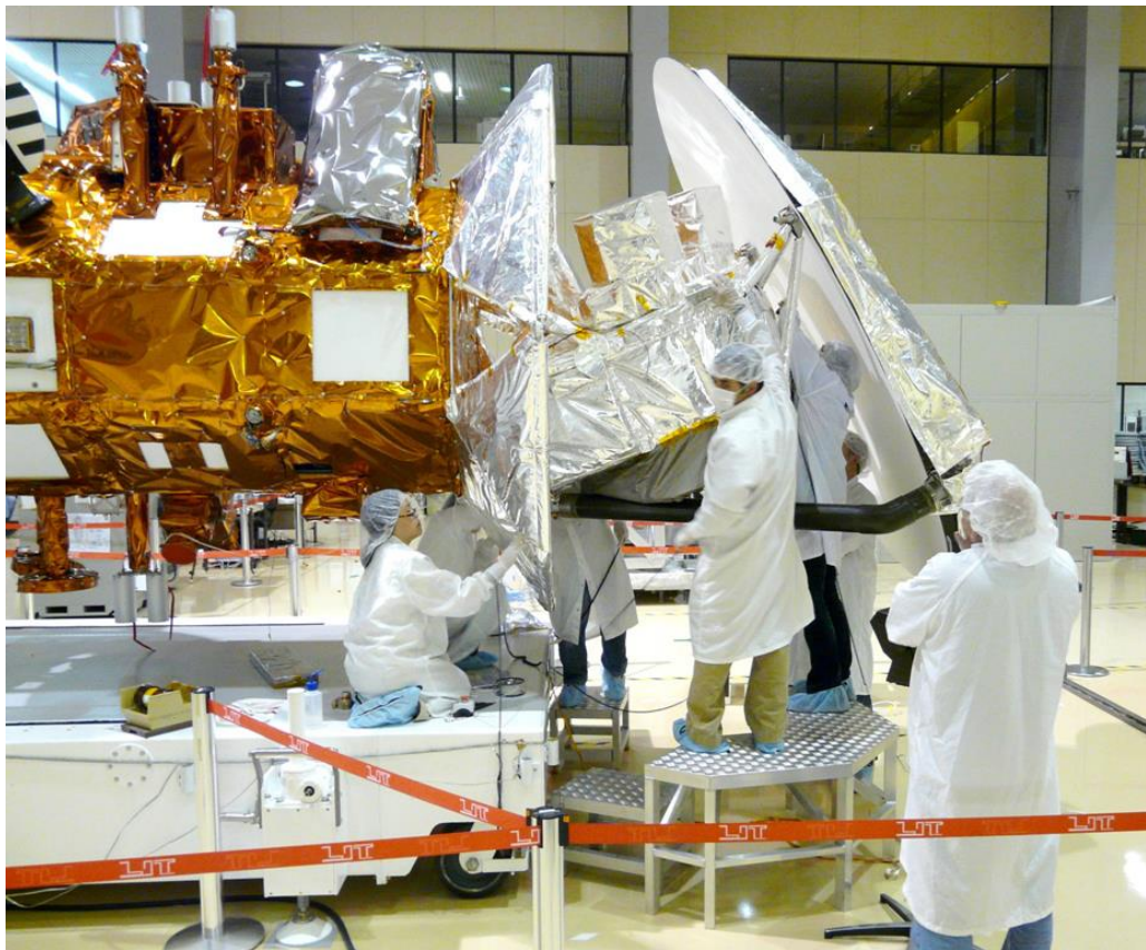
Figure 20: Aquarius satellite covered with Kapton tape and Aluminum film.
