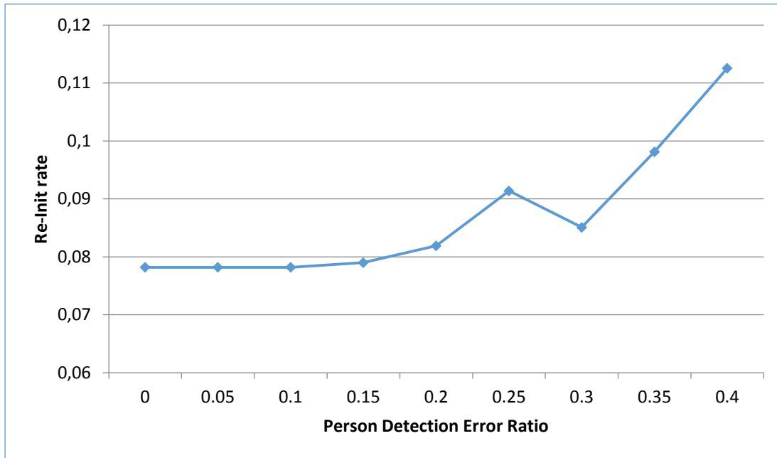
Figure 27. There is no significant change on Re-Init rate with increasing person detection error. Even if increase tendency on Re-Init rate is observed, overall change is less than 0.04% during experiment. This shows us power of CIGT motion modeling.
