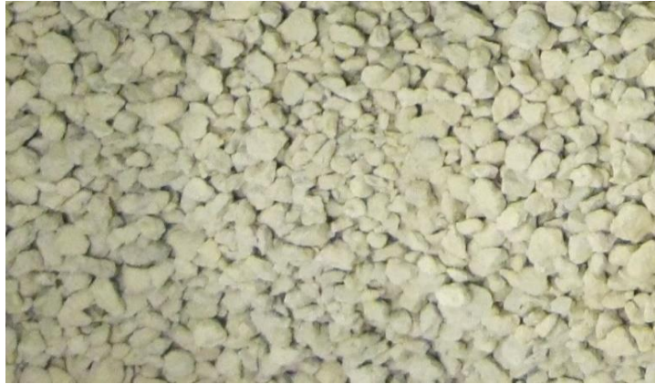
Figure 4.19 : RCA Berlin (8-16 mm in size).
