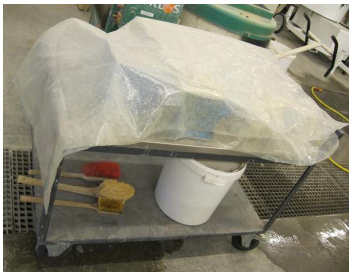
Figure 4.41 : Protection of fresh concrete in the concrete cube moulds.
