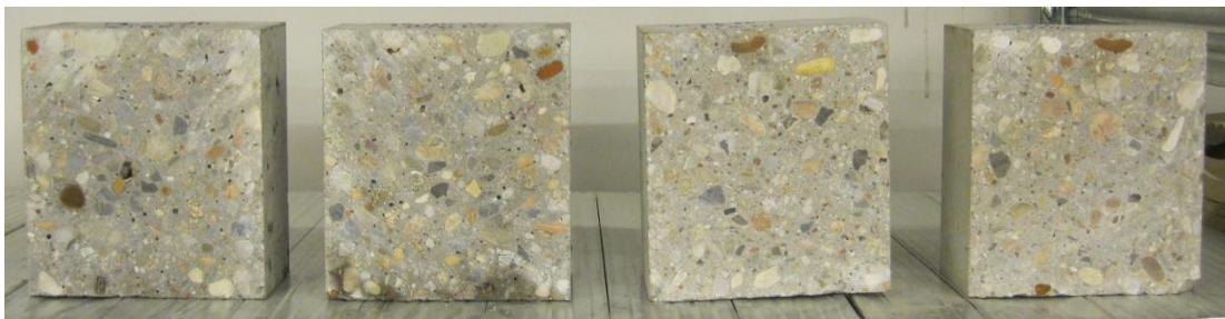
Figure 5.1 : Concrete made with 20 % RCA.
