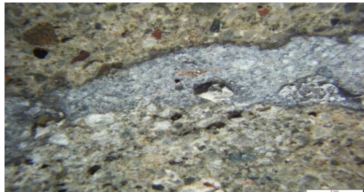
Figure 5.13 : Concrete made with RCA Istanbul at 2 mm length scale.
