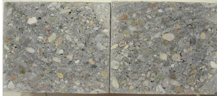
Figure 5.5 : Concrete made with 100% RCA from Berlin.
