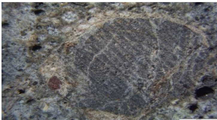
Figure 5.18 : Concrete made with RCA Berlin at 2 mm length scale.
