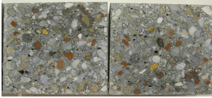
Figure 5.4 : Concrete made with 100% RCA from Istanbul.
