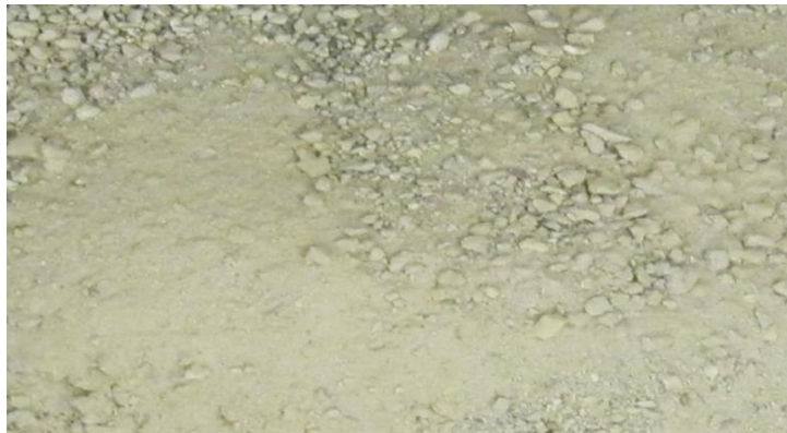
Figure 4.20 : RCA Berlin (2-8 mm in size).
