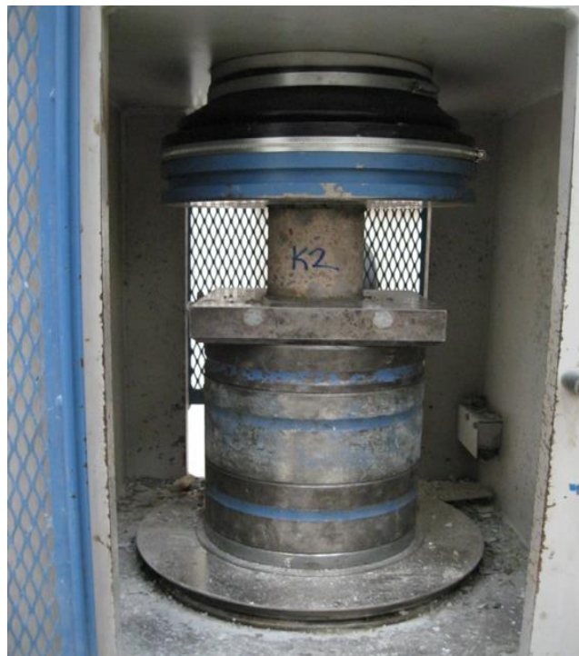
Figure 4.11 : Compressive strength test.
