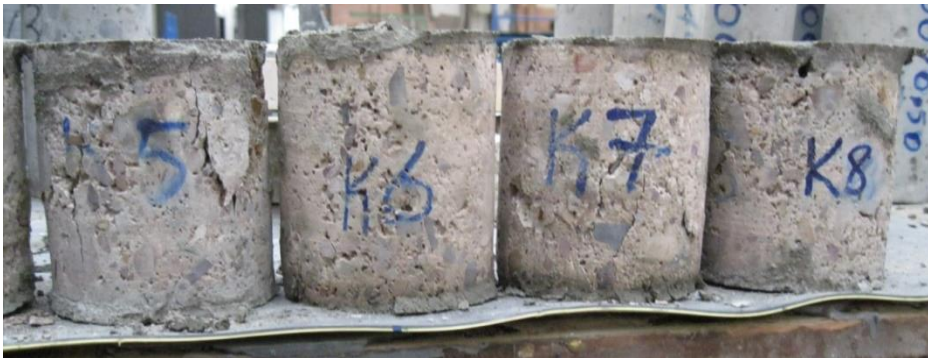
Figure 4.13 : Second group of the core samples after the experiment.
