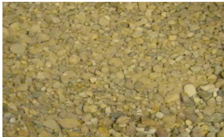
Figure 4.24 : NA (2-8 mm in size).
