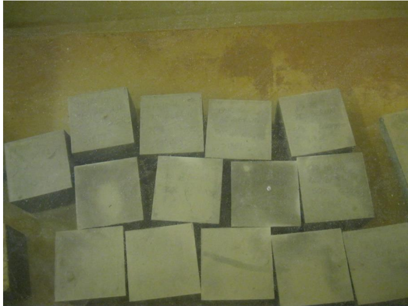
Figure 4.42 : Curing of the concrete specimens for 28 days.
