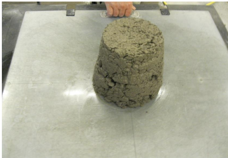
Figure 4.34 : Concrete right after cone was removed.
