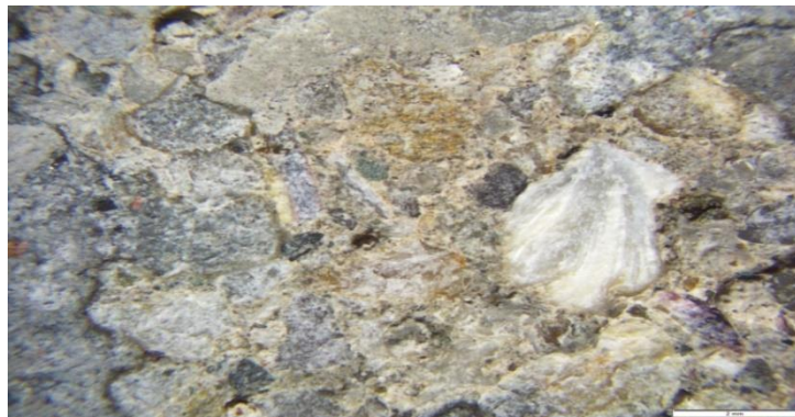
Figure 5.12 : Concrete made with RCA Istanbul at 2 mm length scale.
