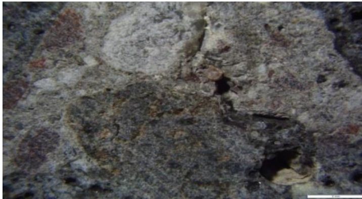
Figure 5.16 : Concrete made with RCA Berlin at 2 mm length scale.
