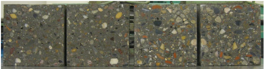
Figure 5.2 : Concrete made with 50 % RCA.
