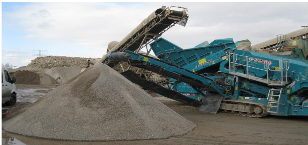
Figure 3.31 : RCA size between 2-8 mm at Arkenberge in Berlin.
