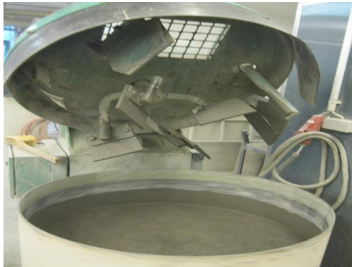
Figure 4.38 : Concrete in the concrete mixer.
