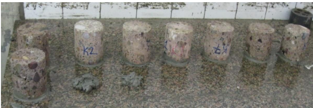
Figure 4.9 : Application of topping to the core samples.
