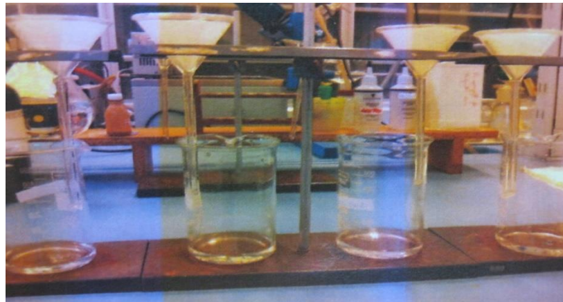
Figure 4.45 : Representation of the filtration of the precipitated barium sulphate.
