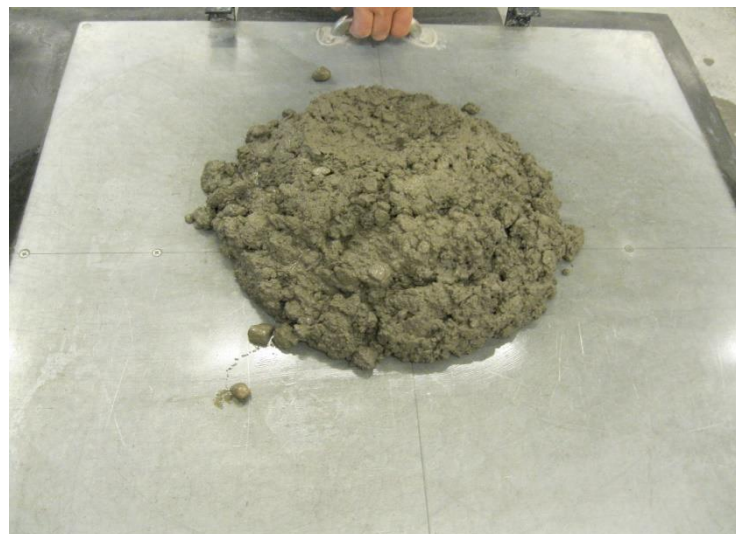
Figure 4.35 : Concrete after the flow table was dropped 25 times.
