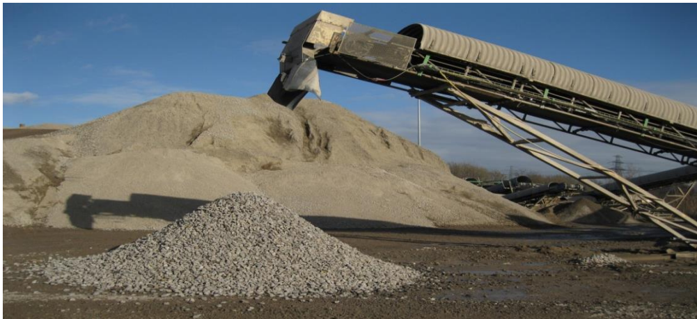
Figure 3.30 : RCA size between 8-16 mm at Arkenberge in Berlin.
