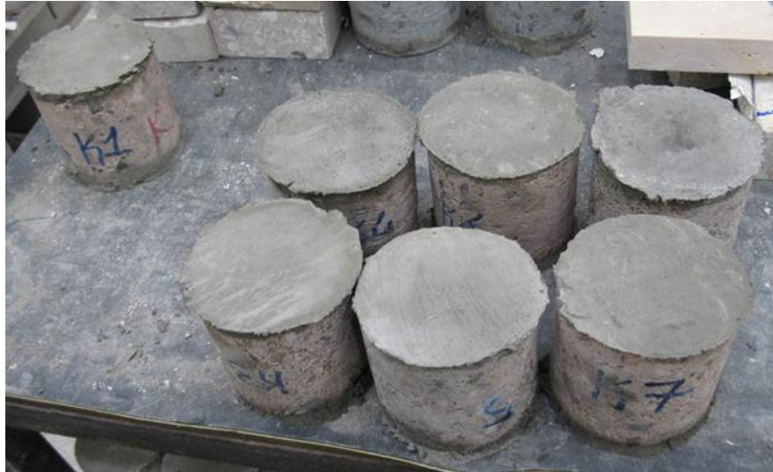
Figure 4.10 : The core samples before compressive strength test.
