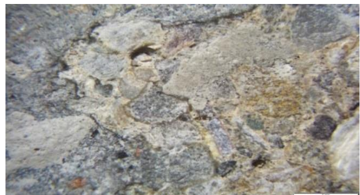
Figure 5.14 : Concrete made with RCA Istanbul at 2 mm length scale.
