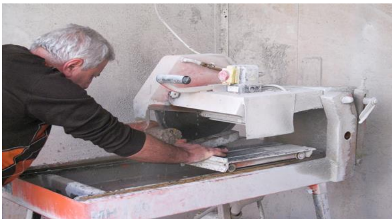
Figure 4.8 : Cutting of uneven ends of the core sample.
