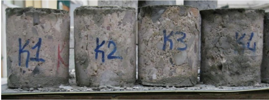
Figure 4.12 : First group of the core samples after the experiment.
