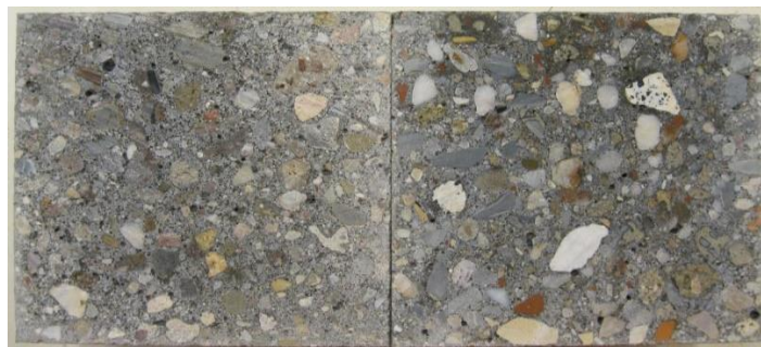
Figure 5.3 : Concrete made with 75% RCA.
