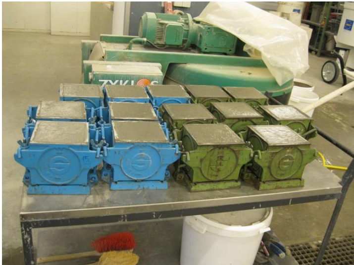
Figure 4.40: The specimens for compressive strength test.
