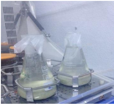
Figure 2.5. Conditioning of clinoptilolite particles with 1 M NaCl.
