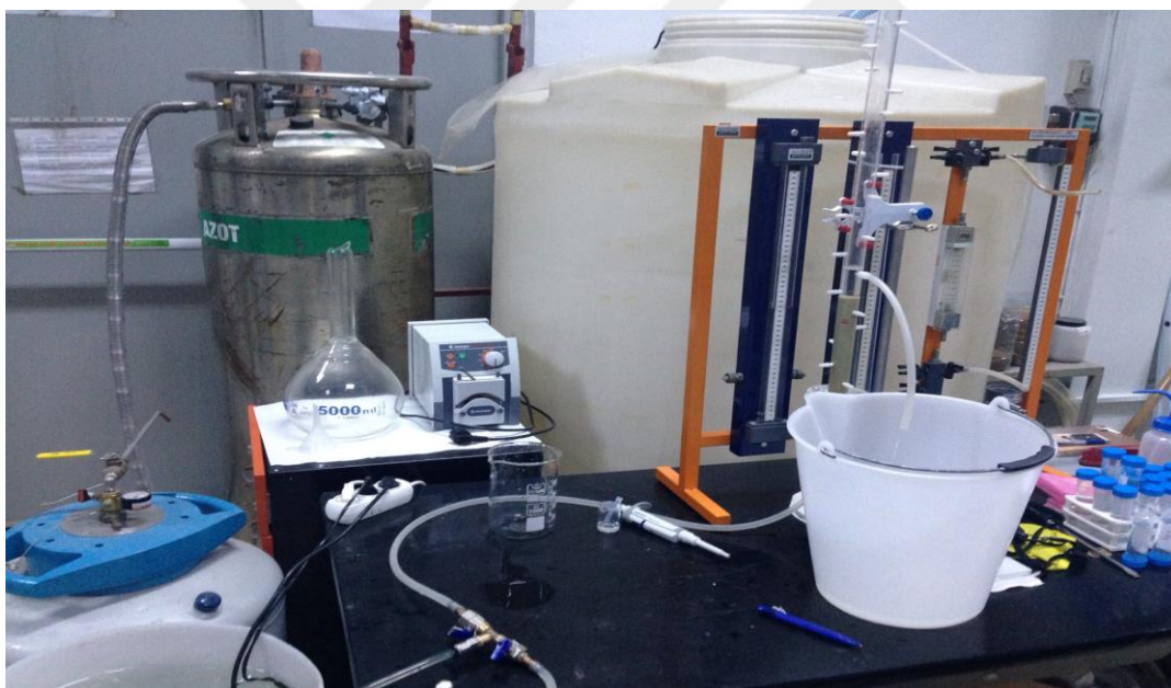
Figure 2.2. Experimental setup used during the fluidized bed ion exchange studies.
